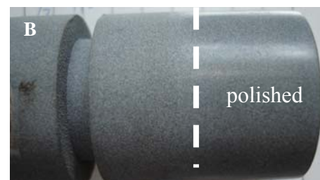
Fig. 4, (A), the microstructure of the coating. (B) the shear pin with Al_2O_3+3\% TiO_2 coating before/after polishing
