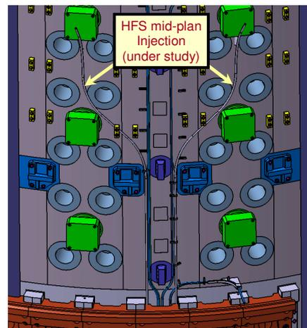
Figure 8 Pellet flight tube layout for HFS midplane injection
