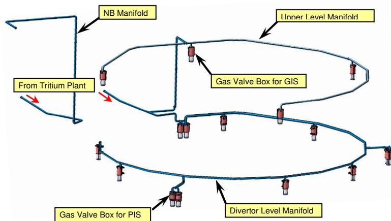
Figure 2 Fuelling manifold layout
