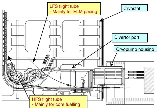
Figure 7 Pellet Flight Tube Layout
