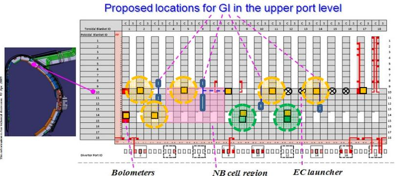
Red boxes are the bolometers, orange the VIS/IR, green the Neutral Particle Analyzer: Interferences are expected in the shaded ellipses.
