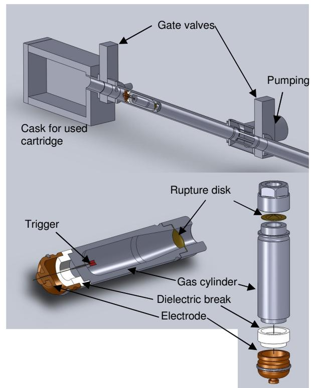
Figure 11 Proposed gas cartridge for MGI DMS
