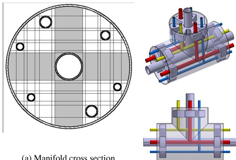
(a) Manifold cross section
