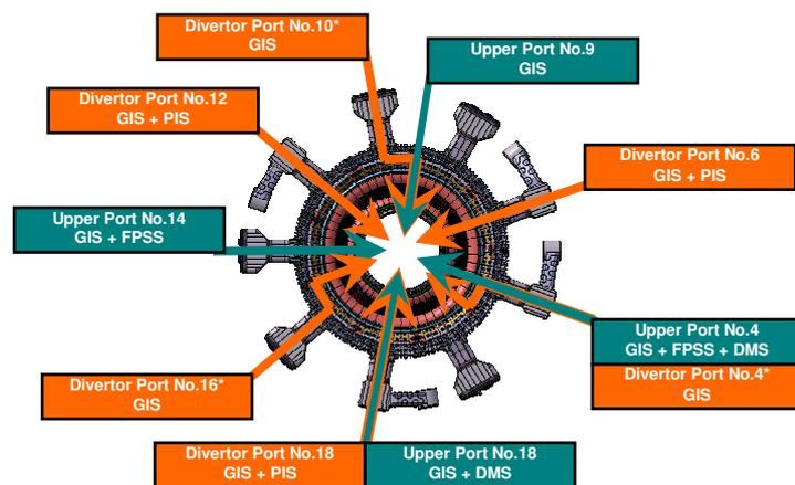
Figure 1 Toroidal distribution of fuelling system
