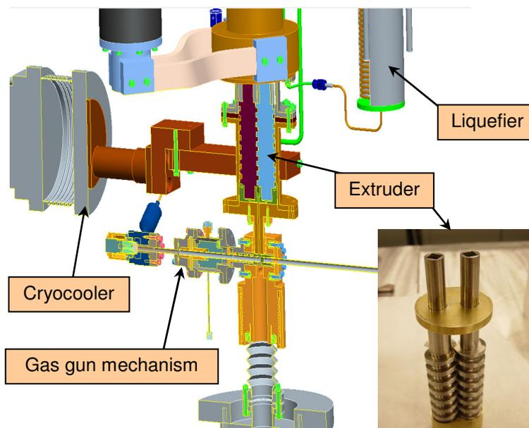
Figure 9 Prototype twin screw extruder
