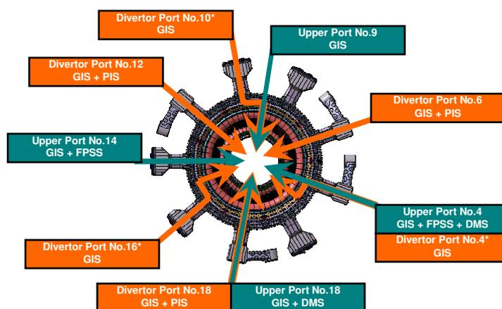
Figure 1 Toroidal distribution of fuelling system
