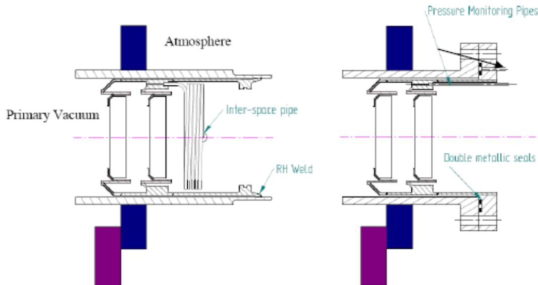
FIG6: Options being considered for the window arrangements. This includes a bolted and welded flange.
