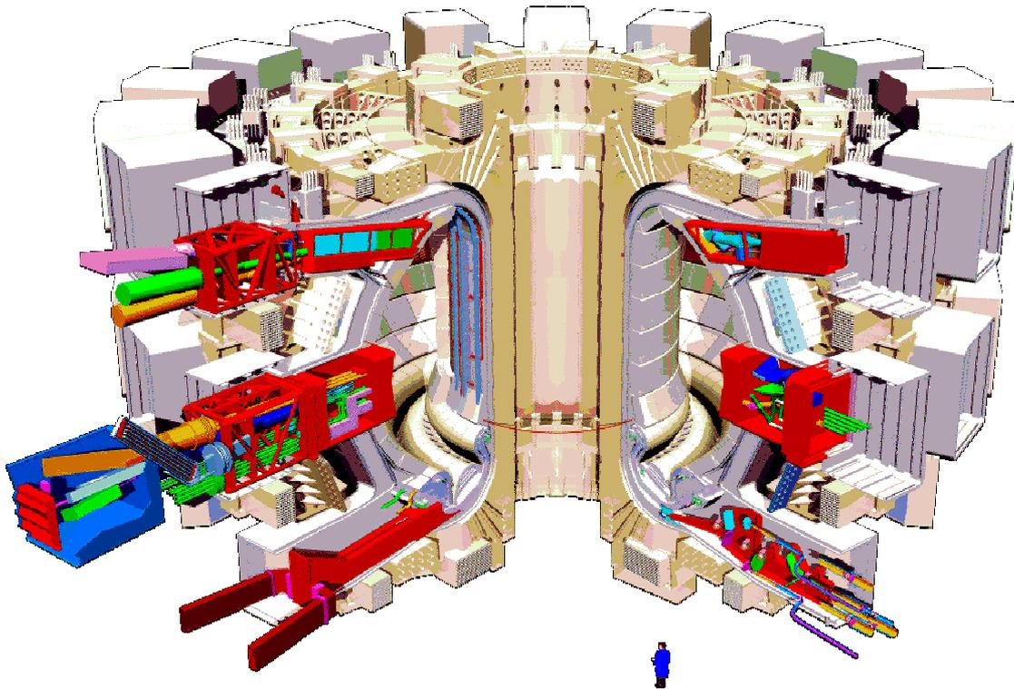
*FIG 1: Cutaway illustration of the ITER device showing the port access at the upper, equatorial and lower areas.*
