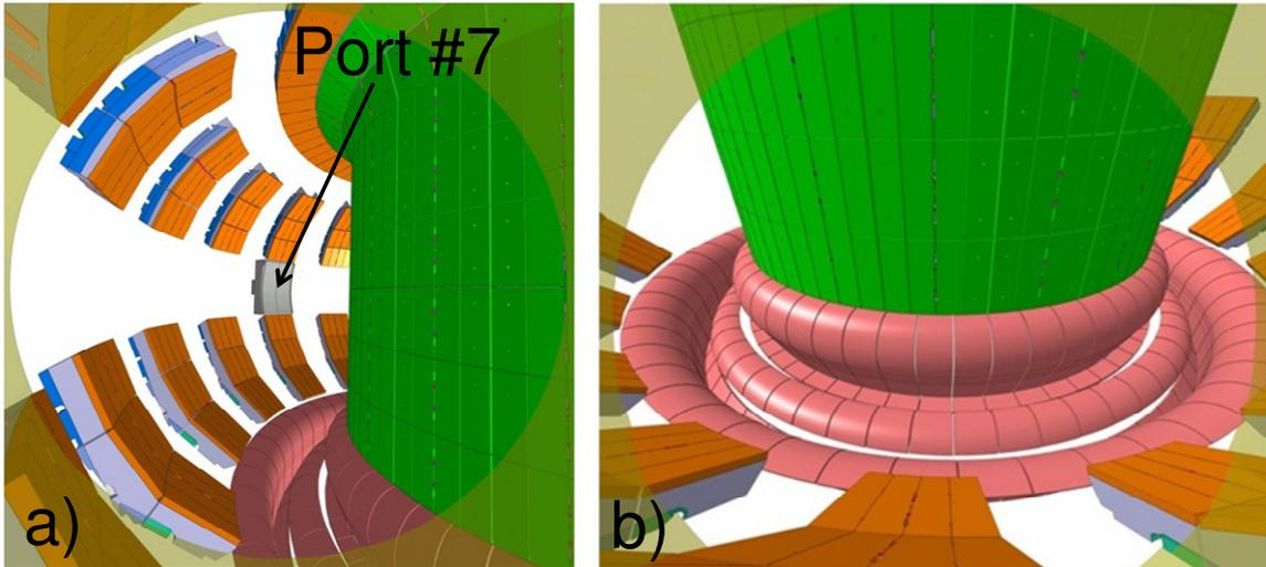
FIG. 3: Views from equ. port # 12: a) left tangential view: equ. port #7 contains a port-plug blanket; b) divertor view.
