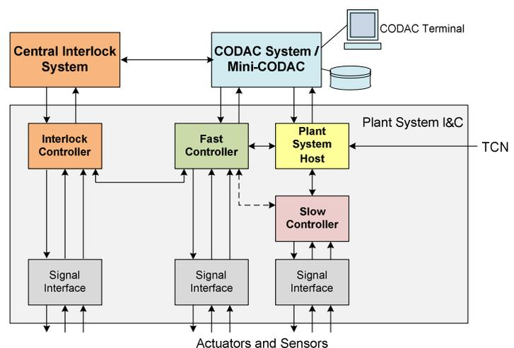
FIG 4: Architecture of central and plant system instrumentation and control including network interfaces.
