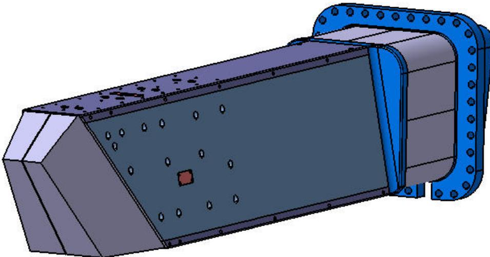
*FIG 2: Structure of upper port plug. The port plug itself is mainly a shell. The inside is taken up by diagnostic systems integrated in robust extractable structures.*
