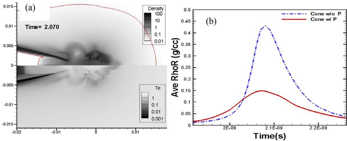
FIG. 3 (a) Mass density contours (top) and electron temperature contours (bottom) at maximum compression time in the implosion of initially perturbed cone-guided shell target. (b) Time history of averaged areal density ( $\rho R$  [ $\text{g}/\text{cm}^2$ ]). An unperturbed initial target case (Dot-dash line), and perturbed initial target case (solid line).
