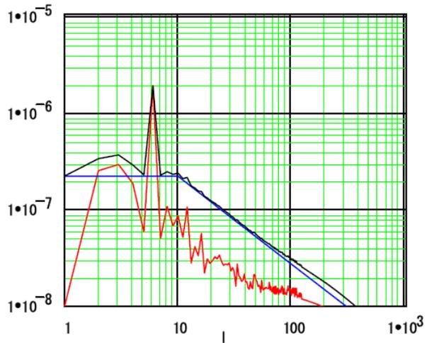
FIG. 2. Amplitude of initial target surface perturbation. Red line (“measured” line) indicates a typical target roughness. The measured imprint is modeled and imposed on the target surface roughness, of which amplitude is indicated as blue line (“imprint model” line). The sum of these amplitudes is indicated as black line (“total” line).
