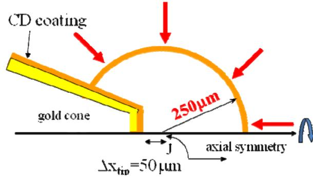
FIG. 1. Configuration of target, which is typical size and materials for GXII experiment. Thickness of the tip is 8  $\mu\text{m}$ , and opening angle of the cone is 30 degree.
