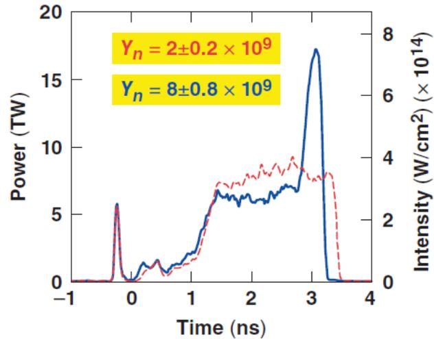
FIG. 7: Comparison of “standard” (red) and shock ignition (blue) pulse shapes used in OMEGA experiments. [18]
