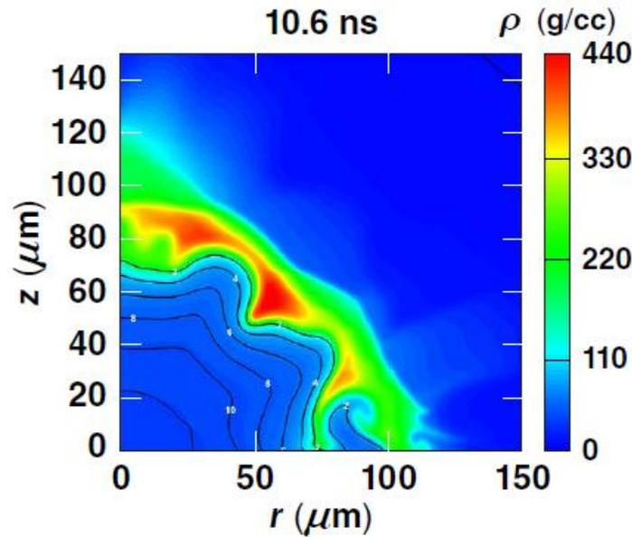
FIG. 1: Two dimensional simulation predictions of the density of a compressed Polar Drive target near peak compression of a target that produces a gain of 18 on the NIF.
