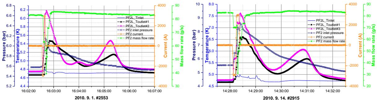
FIG. 8. Temperature rise of PF2L in single coil test (left) and simultaneous coil test (right)
