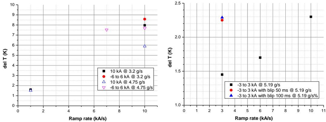
FIG. 7. Relationship between current ramp rate and temperature rise in PF1L (left) and PF2L (right)
