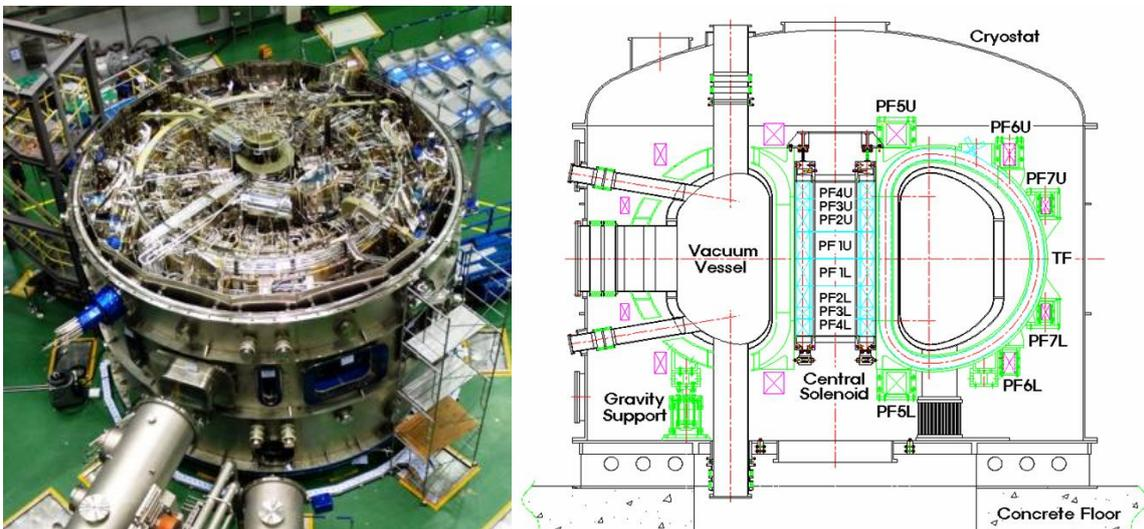
FIG.2. KSTAR magnet system
