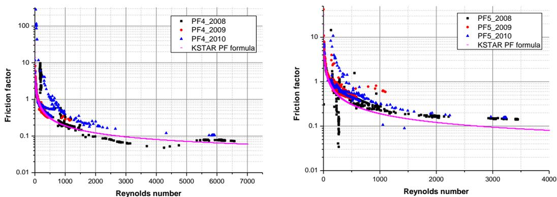
FIG. 4. Friction factor of PF4 (left) and PF5 (right)
