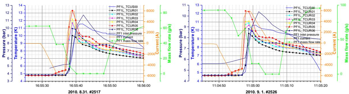
FIG. 6. Temperature rise of PF1L in normal mass flow (left) and increased mass flow (right)
