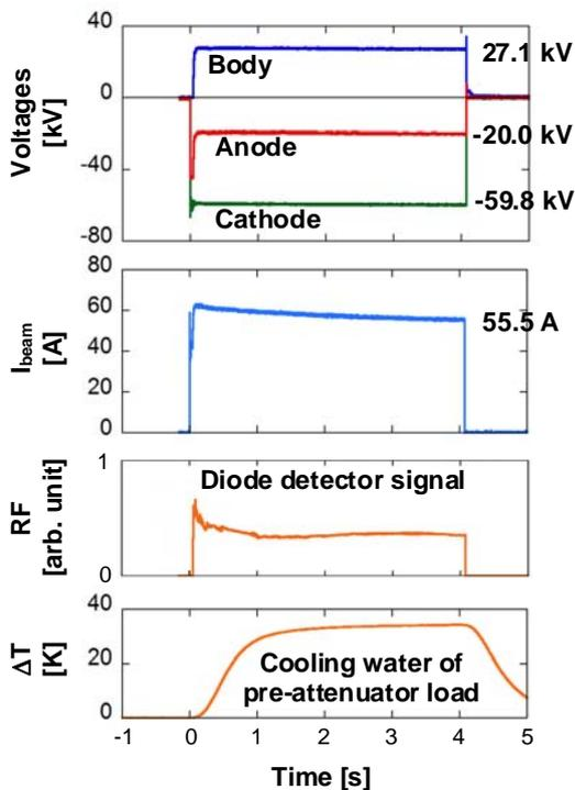
FIG. 6. Temporal evolutions of the applied voltages, beam current, RF signal detected by a diode detector at the miter bend and temperature rise of the cooling water for the pre-attenuator dummy load on the oscillation of 1.5 MW for 4 s.
