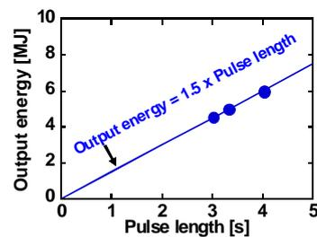
FIG. 7. Output energy of the gyrotron and pulse length. Straight line shows the expected energy at the output power of 1.5 MW.
