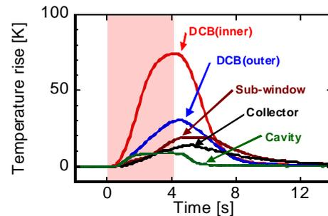
FIG. 10. Temporal evolution of temperature rise of the coolant water for the dc-break (inner and outer), sub-window, collector and cavity.
