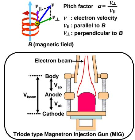
FIG. 3. Schematic view of a triode type magnetron injection gun and the definition of the pitch factor.
