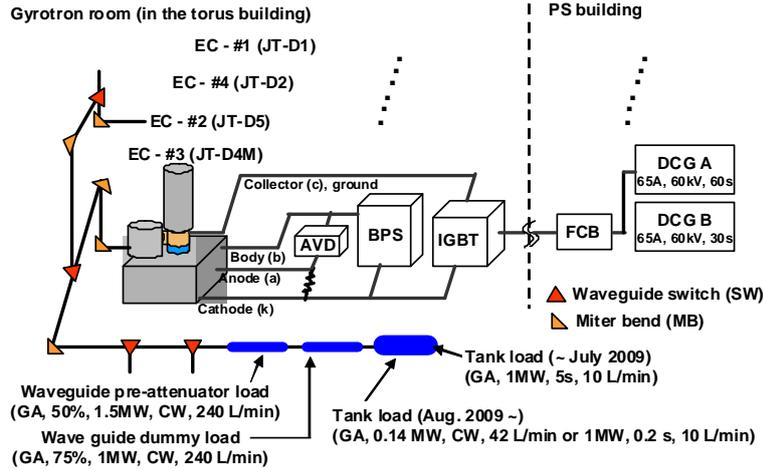
FIG. 1. Schematic view of the JT-60 ECRF system for high power and long pulse experiments. The EC-#2 was used for the high power operation and the EC-#3 was used for long pulse operation with improved gyrotron.
