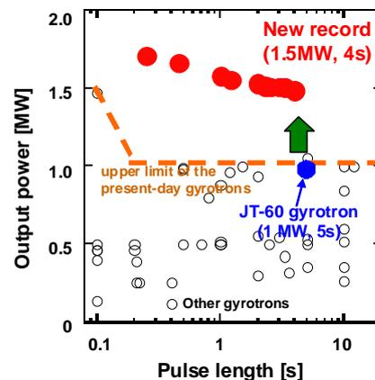
FIG. 8. Progress on the high power gyrotron oscillation achieved by the JT-60 gyrotron (closed circles) and other gyrotrons (open circles) in the world (before 2008).
