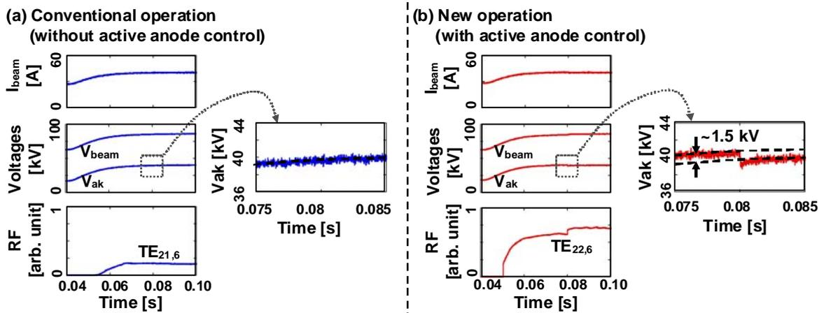
FIG. 4. Typical waveforms of (a) conventional operation and (b) new operation technique. All operation parameters were fixed except the small difference in the  $V_{ak}$  at the beginning of the pulse. The start up condition of the target mode of TE<sub>22,6</sub> is satisfied by increasing  $V_{ak}$  by  $\sim 1.5$  kV. Once the target mode excited, the target mode is maintained even the  $V_{ak}$  was reduced at  $t = 80$  ms.
