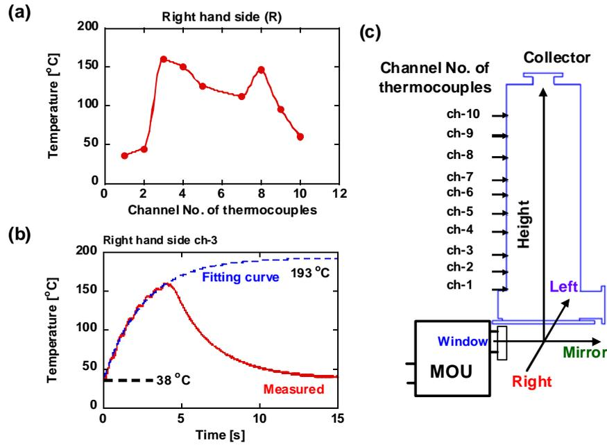
FIG. 9. (a) Spatial distribution of the collector temperature at the right hand side of the collector (seeing from the MOU side) measured with thermocouples installed at the middle of the inner and cooled surfaces of the collector in depth and (b) the time evolution at ch-3 of an oscillation at 1.5 MW for 4 s. The position of the thermocouples, ch-1 ~ ch-10, are also shown in (c).
