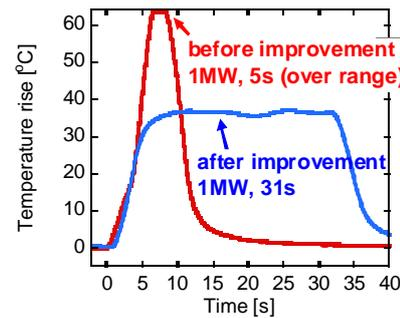
FIG. 11. Temporal evolution of the coolant water for the DC-break before and after improvement of the mode converter.
