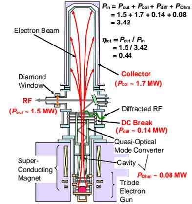
FIG. 2. Structure of the JT-60 gyrotron and an example of the heat load for an output power of 1.5 MW of a gyrotron.
