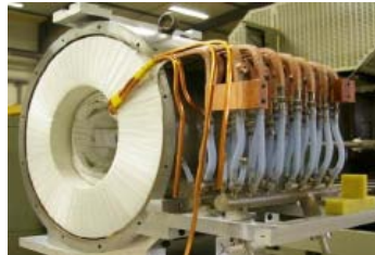
Figure 3: One solenoid of the injector under magnetic measurement
