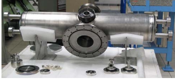
Figure 5: One of the two Half-Wave Resonator prototypes (“naked” cavity) of the SRF Linac
