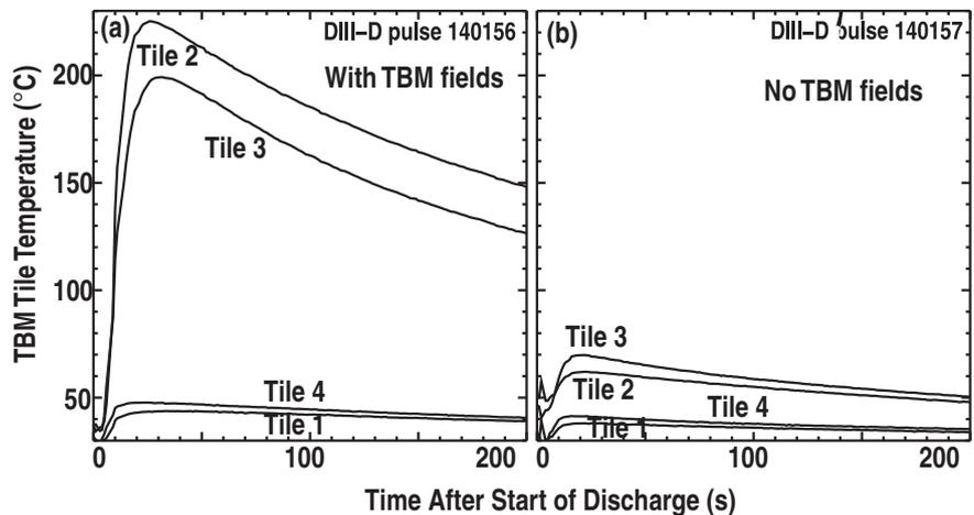
FIG. 2. Tile temperatures measured with the thermocouple at the back of the carbon tiles for two similar DIII-D discharges. In (a) the TBM fields were present while in (b) they were not present.
