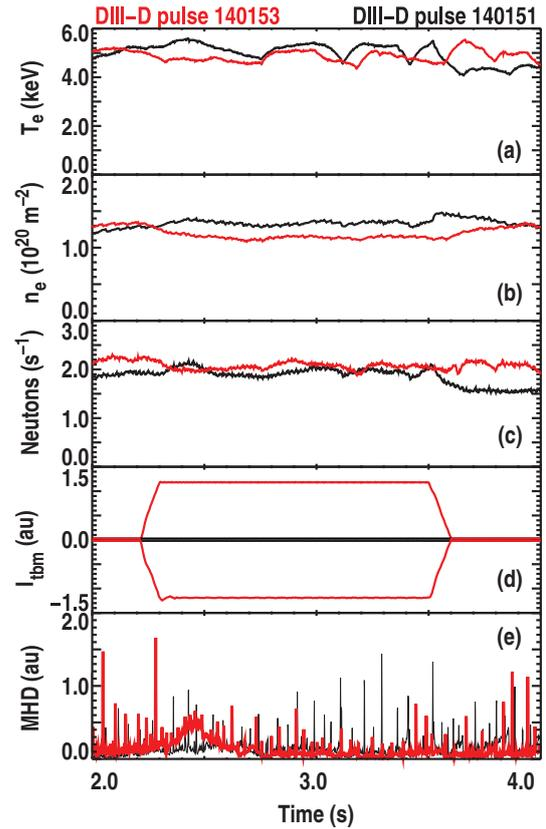
FIG. 3. The central electron temperature (a), density (b), neutron rate (c), TBM coil currents (d), and MHD activity (e) for a discharge without TBM fields in black (pulse 140151) and one with the TBM fields engaged in red (pulse 140153).
