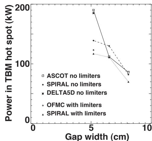
FIG. 6. Hot spot power induced by the TBM fields versus the gap width calculated with various codes.
