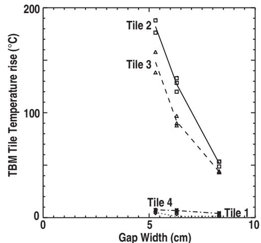
FIG. 4. The measured thermocouple temperature rise at the back of of the four tiles for a 1 s long TBM pulse versus the outer gap width. Each symbol is a separate discharge.
