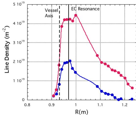
Fig.3 Line Density profiles for two different injection toroidal angles:  $0^\circ$  (blue) and  $20^\circ$  (red) at 3 ms after switch on of 0.4 MW of EC power. Pre filling pressure 4.6 mP.
