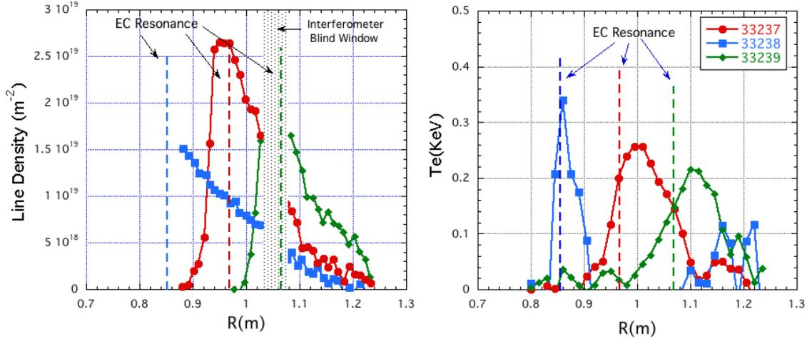
Fig.7 (left) Line density profiles versus major radius taken 5ms after 0.4MW of EC switch on for different resonance positions (dotted lines). The gray region is the blind window of  $CO_2$  interferometer. (right) Electron temperature profiles from ECE-Michelson taken at 50 ms.
