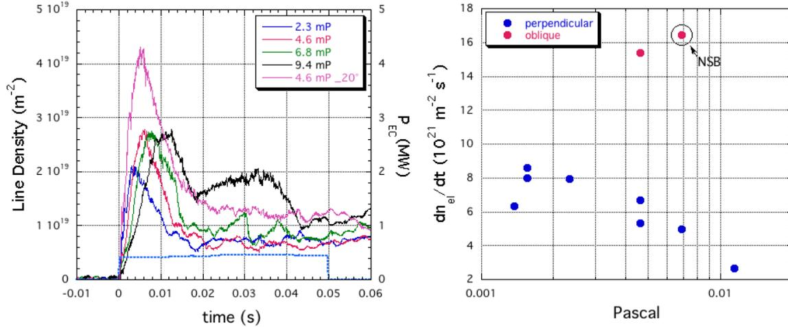
Fig.2 (left) Central line density evolution at different pressures. EC power is on right scale, in all cases toroidal angle is  $0^\circ$  except for the magenta one ( $20^\circ$  of oblique injection); electric field is 1.5 V/m and  $B_0=5.3T$ . (right) Max of  $n_{ei}$  time derivative as a function of pressure. Blue points refer at  $0^\circ$  and sustained breakdown. Red points for  $20^\circ$  of oblique injection, for the circled one sustained breakdown has not been achieved.
