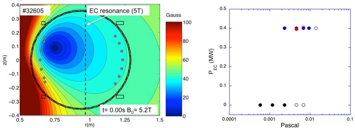
Fig.1: Left: FTU poloidal field at 0.0s. Toroidal and poloidal limiter together with the position of the EC resonance are shown. Right: Pressure scan for EC injected power; open circle: Not Sustained Breakdown, close circle: Sustained Breakdown. In blu perpendicular injections ( $0^\circ$ ) in red oblique ( $20^\circ$ ), in black pure ohmic cases.
