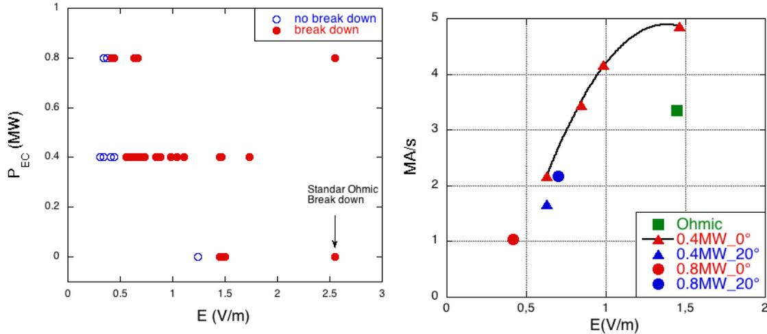
Fig.4 (left) FTU results for break down as function of electric field and EC power. (right)  $I_p$  derivative vs Electric field in different conditions of EC assisted break down. Pulse length is 200ms and pressure below 2 mP.
