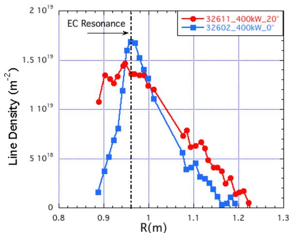
Fig.5 Line Density profiles measured 1 ms after EC switch on for 0° and 20° of injection angles.
