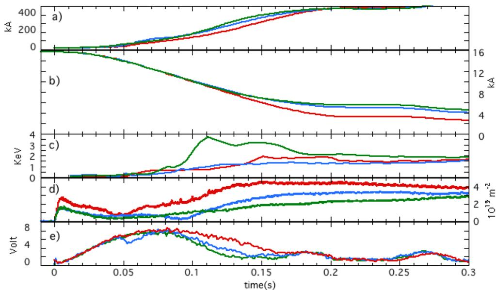
Fig.8 Time evolution of a) plasma current, b) ohmic transformer current, c) central electron temperature, d) line density at EC resonance major radius and e) loop voltage. Red lines refer to #33237 with  $R_0 - R_{EC} = +2cm$ ; blue lines to #33238 with  $R_0 - R_{EC} = +12cm$  and green lines to #33239 with  $R_0 - R_{EC} = -14 cm$ . ECRH power are switched on at 0s with perpendicular injection.
