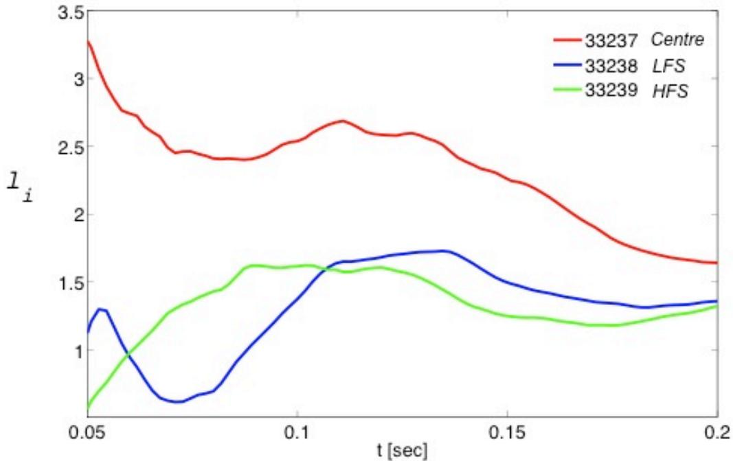
Fig 9. Evolution of internal inductance (normalized to  $\mu_0 R$ ) calculated from ODIN reconstruction data and experimental pressure profiles. The line colours refer to different  $R_{EC}$  (the same of fig.8).
