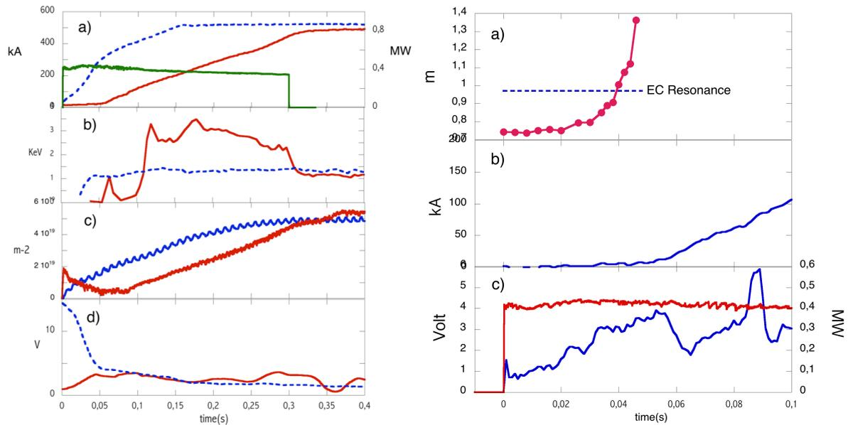
Fig.6 (left) Comparison between Ohmic startup (#32590, dotted blue) and a low E field EC assisted one (#32602, solid red): a) plasma currents and EC power (green), b) central Te, c) central line density, d) Vloop. (right) First 100 ms of the same shot. a) centre of the null evolution, b) plasma current, c) EC power (red line) and loop voltage (blue line).
