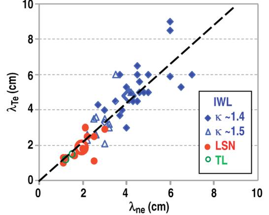
FIG. 2. Correlation between density and temperature e-folding lengths.
