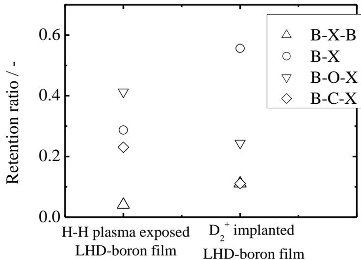
Fig. 3 The hydrogen isotopes retention ratio as each desorption peak in H-H main plasma exposed and  $D_2^+$  implanted LHD-boron film. (X means hydrogen isotopes)
