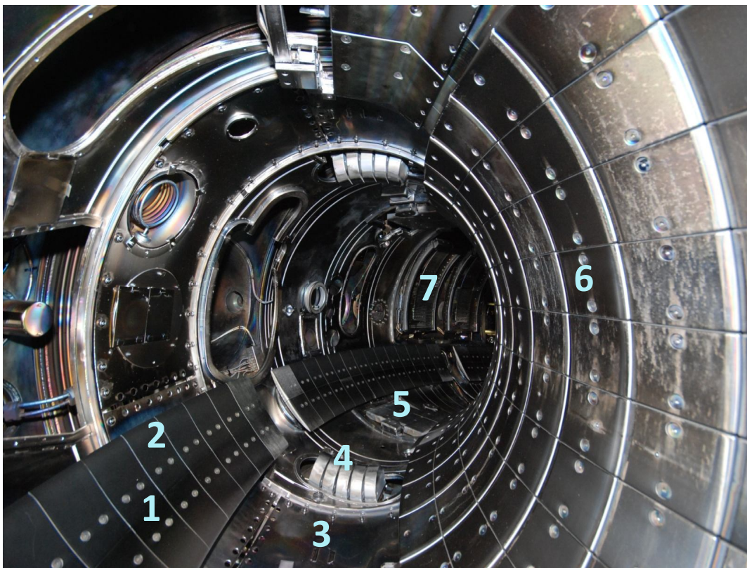
Fig. 1. Sampling of dust in TEXTOR: deposition (1) and erosion (2) zones on ALT-II; bottom of the Inconel liner (3), main poloidal limiter (4), DED bottom shield (5), inner bumper limiter (6), ICRF antenna (7).
