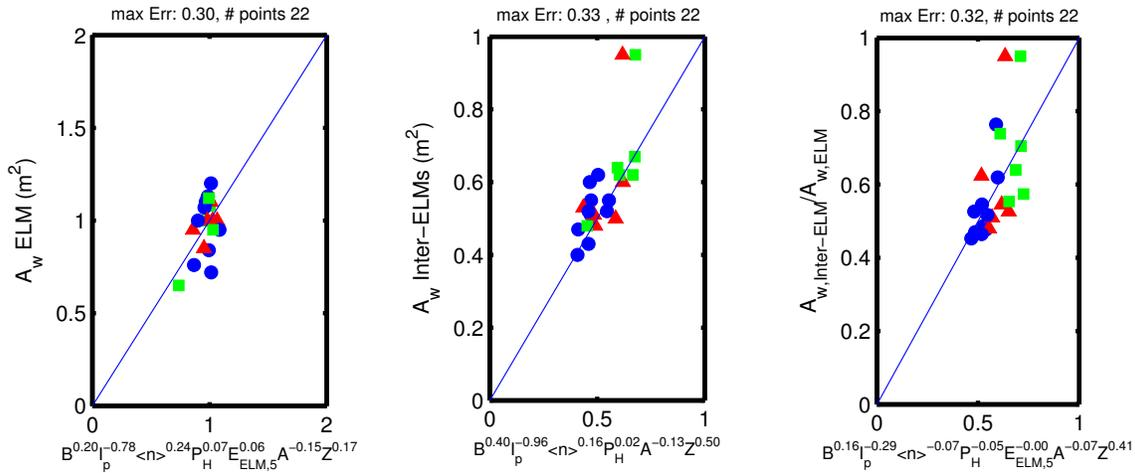
Figure 5: IR-measured wetted areas,  $A_w [m^2]$ , during ELM (left), inter-ELM (middle) and their ratio (right) vs best-fit scalings with field, current, density, heating power, A and Z (and for ELM quantities also with ELM deposited energy) for all ion species.
