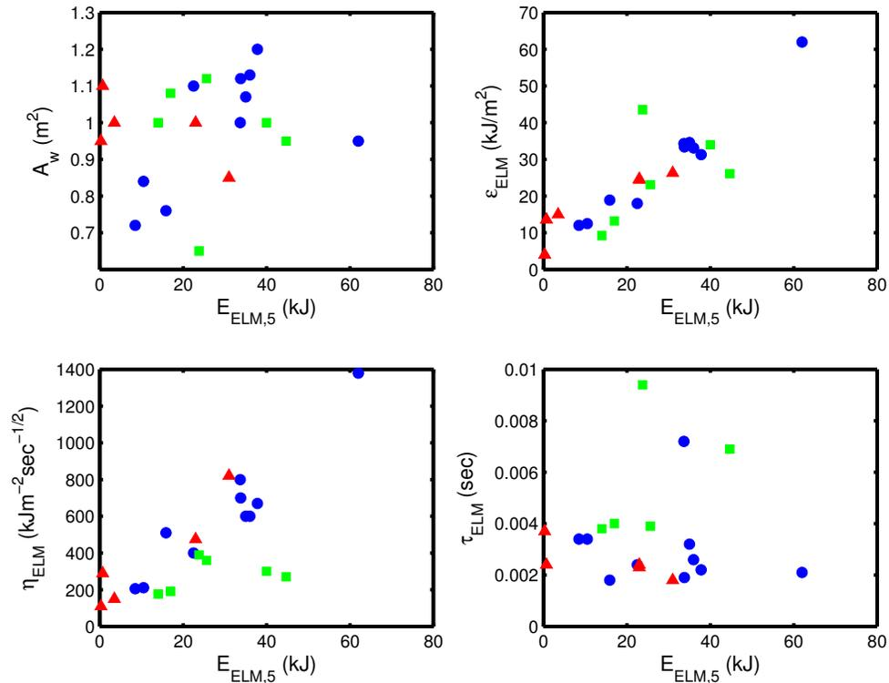
Figure 6: ELM wetted area (top left), maximum ELM energy load (top right) and ELM impact factor (bottom left) and ELM deposition time scale (bottom right) vs ELM deposited energy (kJ).
