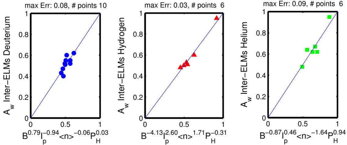
Figure 4: IR-measured inter-ELM wetted areas,  $A_w^{inter-ELM} [m^2]$  vs best-fit scaling with field, current, density and heating power, for D (left), H (middle) and He (right) plasmas. Note that due to insufficient number of data points (6 points vs 4 scaling variables), clustering in a small range, the stand alone scalings for H and He are unreliable.
