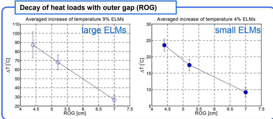
Figure 2: ELM heat load interaction with outer limiter for two D discharges, with relative ELM size, ( $\Delta W_{ELM}/W_{dia}$ ) of 9% (left) and 4% (right), for different values of the outer gap (ROG)
