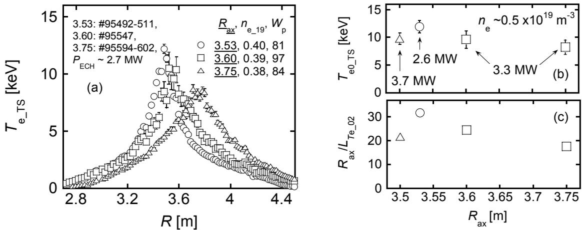
FIG. 3. (a) the radial profiles of  $T_e$  for three configuration cases;  $(R_{ax}, B_0) = (3.53 \text{ m}, 2.705 \text{ T})$ ,  $(3.60 \text{ m}, 2.705 \text{ T})$  and  $(3.75 \text{ m}, 2.75 \text{ T})$ , the configuration dependence of (b) the central electron temperature  $T_{e0}$  and (c)  $R_{ax}/L_{Te}$ .
