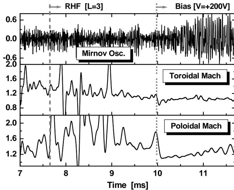
**FIG. 5.** Time evolution of Mirnov oscillation and Poloidal and toroidal Mach Number With RHF (L=3) applied in 7.7 ms and 200V positive limiter Biasing applied in 10 ms.
