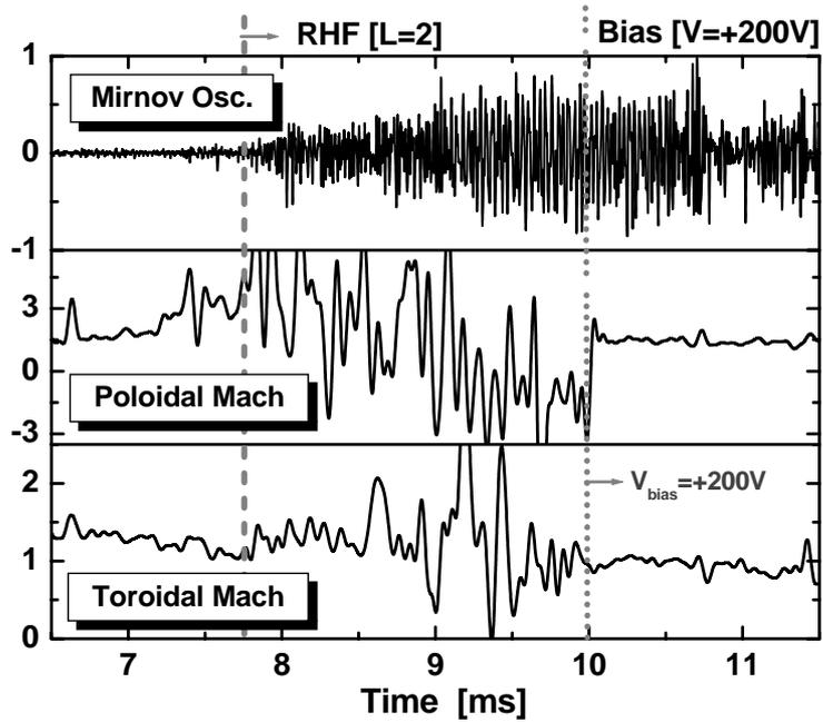
**FIG. 4.** Time evolution of Mirnov oscillation and Poloidal and toroidal Mach Number With RHF (L=2) applied in 7.8 ms and 200V positive limiter Biasing applied in 10 ms.
