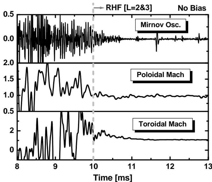
**FIG. 3.** Time evolution of Mirnov oscillation and poloidal and toroidal Mach number with RHF (L=2&3) applied in 10 ms and without biasing.
