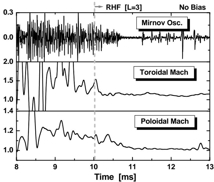
**FIG. 2.** Time evolution of Mirnov oscillation and poloidal and toroidal Mach number with RHF (L=3) applied in 10 ms and without biasing.
