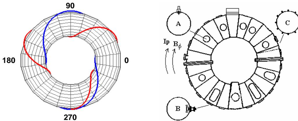
**FIG.1.** Schematic drawing of IR-T1 (Right), locations of Mirnov coils indicated by (C), limiter/electrode biasing position indicated by (B) and 4-pin Mach probe indicated by (A), and typical schematic of  $L=2/1$  and  $L=3/1$  RHF winding coil around the chamber (Left).
