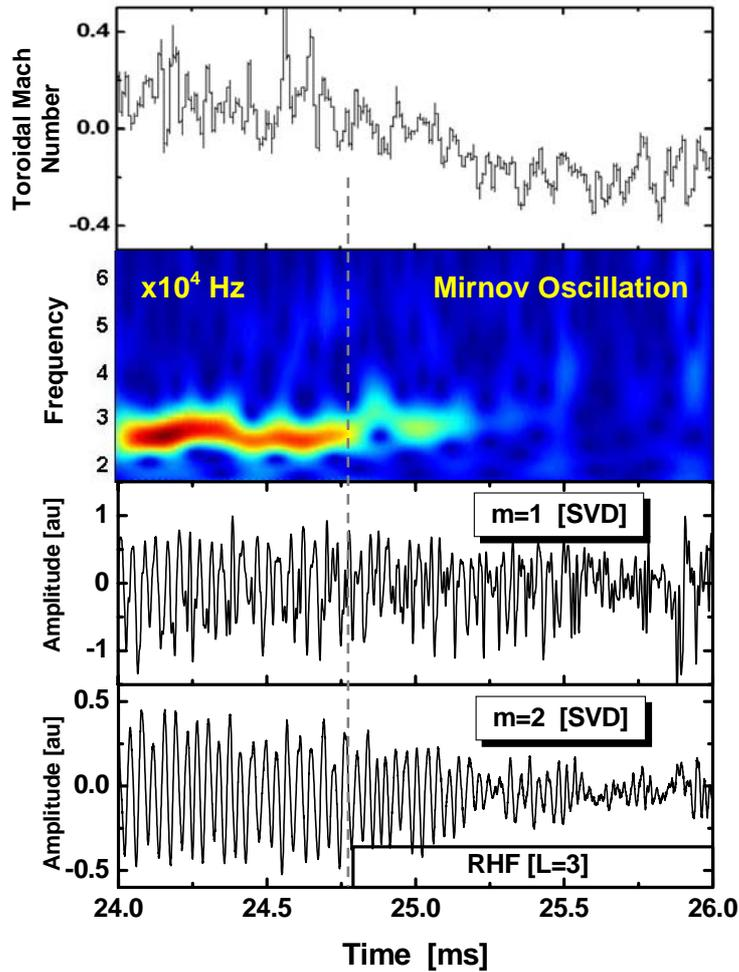
**FIG. 6.** time evolution of plasma behavior during RHF ( $L=3$ ) application in 24.8 ms. The data from toroidal mach number by 4-pin Mach probe, Wavelet spectrum of Mirnov Coil and SVD (0.5ms time intervals) analyses; top to bottom respectively.
