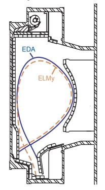
FIG 1: Examples of equilibria used to obtain EDA (blue solid) and ELMy (orange dashed) H-modes
