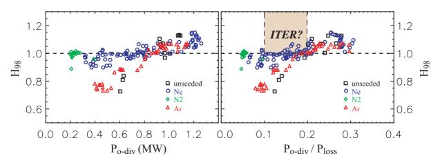
FIG 5: Low-Z impurity seeding of EDA H-modes demonstrates the capability to reduce power to the outer divertor by a substantial factor, while maintaining  $H_{98}$ ~1.(a)  $H_{98}$  vs.power to the outer divertor. (b)  $H_{98}$  vs. the fraction of loss power (approx. equal to input power) falling on the outer divertor. A critical question is whether ITER can operate within the pink box.
