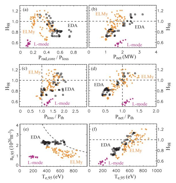
FIG 2: Confinement in L-mode and EDA, ELMy H-modes with intrinsic impurity content only, as a function of (a)  $P_{rad,core}/P_{loss}$ , (b)  $P_{neb}$ , (c)  $P_{loss}/P_{th}$ , (d)  $P_{net}/P_{th}$  and (f) pedestal  $T_e$ . Pedestal  $n_e$  and  $T_e$  are shown in (e) along with a dashed curve representing a constant electron pressure.
