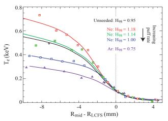
FIG 4. Examples of temperature pedestals without seeding and with impurity seeding from Ne and Ar.
