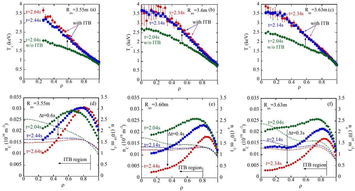
FIG.3. Radial profile of ion temperature in the plasma with (a)  $R_{ax}=3.55\text{m}$ , (b)  $3.6\text{m}$ , and (c)  $3.63\text{m}$ . Radial profile of carbon density in the plasma with (d)  $R_{ax}=3.55\text{m}$ , (e)  $3.6\text{m}$ , and (f)  $3.63\text{m}$ . Dashed lines in (d)-(f) shows the fitted line of electron density profile.
