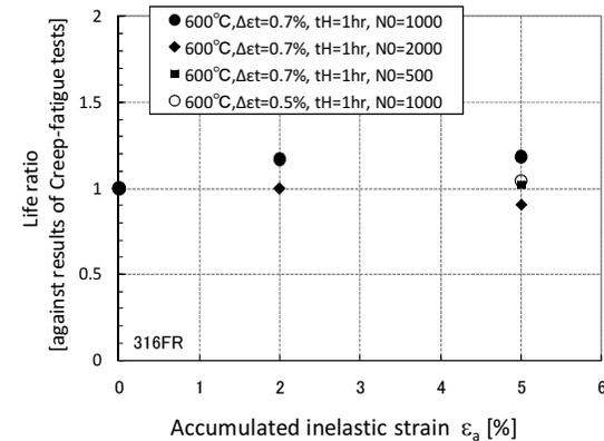
Strength reduction is small in creep-fatigue + ratchet tests compared with fatigue + ratchet ones. From the later results, allowable strain limit is determined as 2%.
