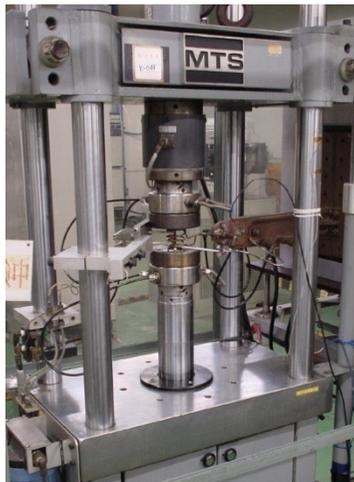
Simulated loading of reactor vessels
