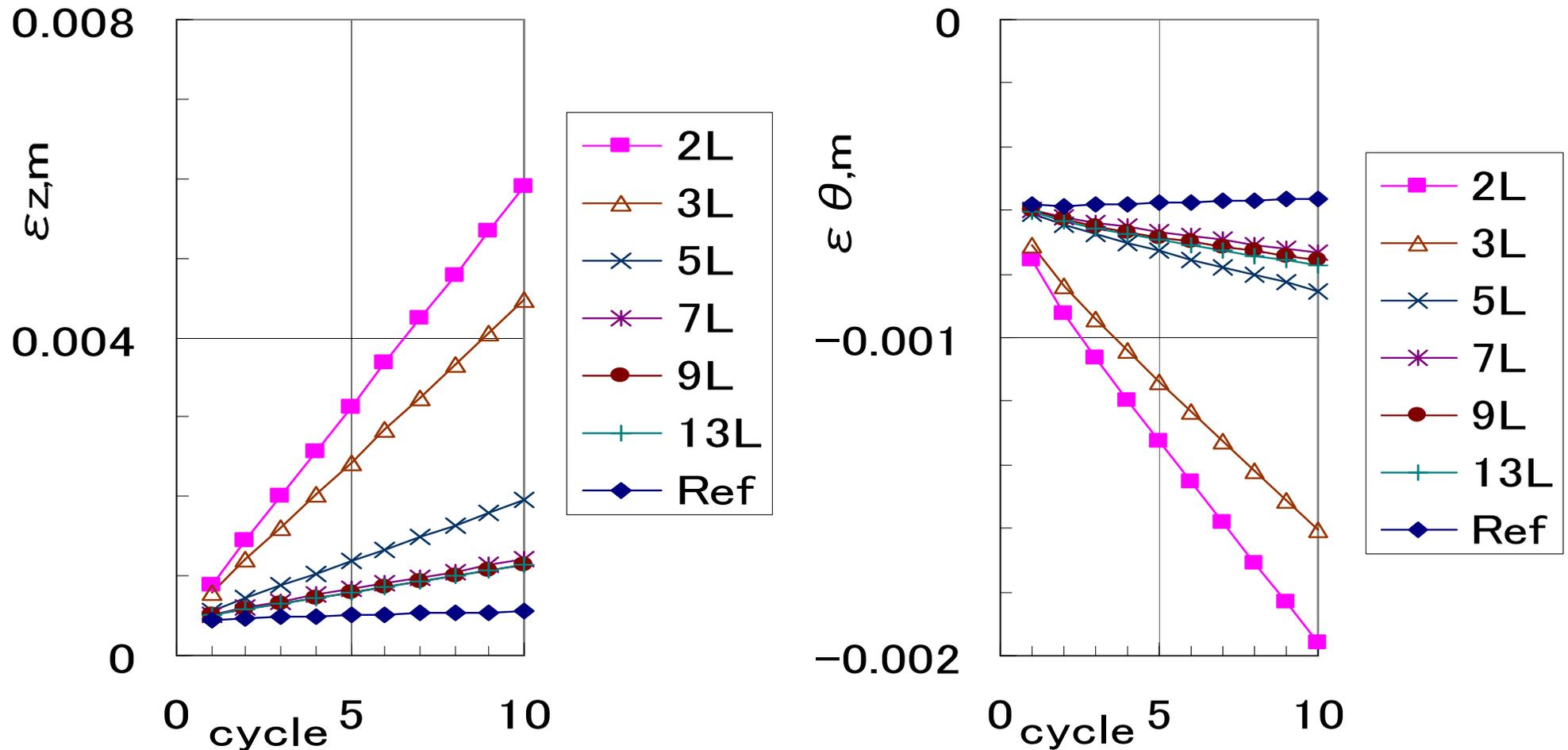
Strain behaviour by MK-SRR model with various number of multi-linear approximation
