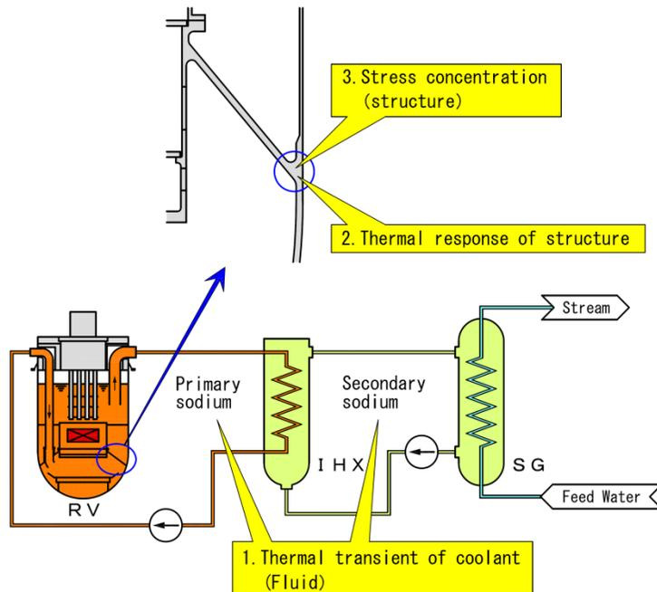
Thermal loads induced by thermal-hydraulic and structural phenomena
