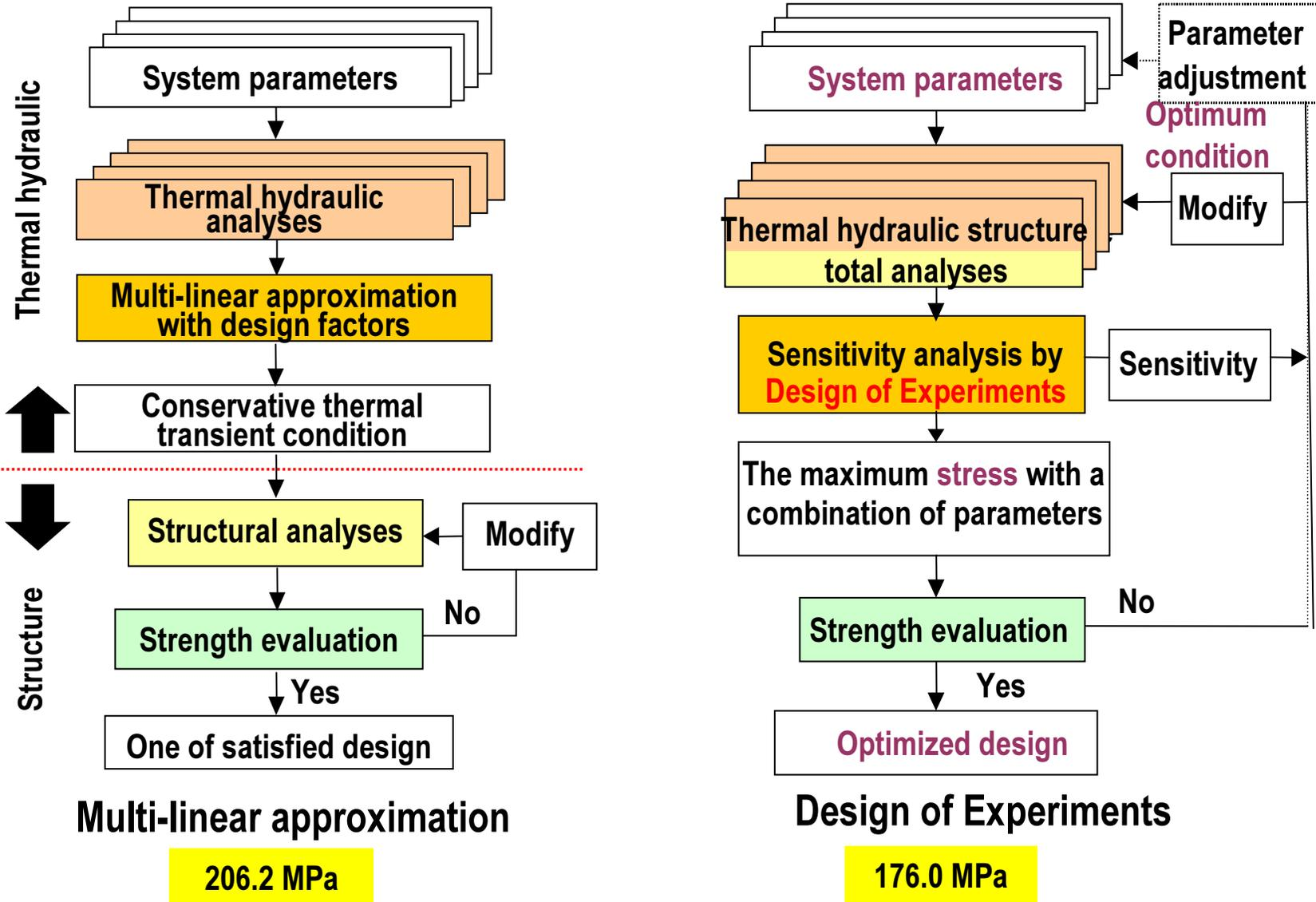
Example prediction of thermal stress at the wall of upper part of reactor vessel
