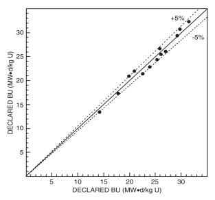
FIG. 1. Operator declared BU compared with the calculated BU values based on the <sup>137</sup>Cs activity measurements.
