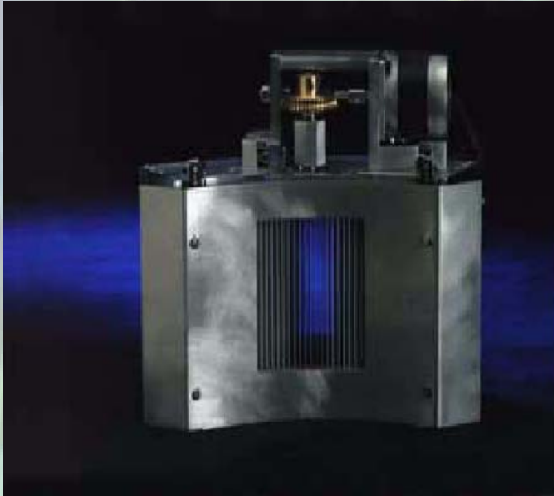
elastically bent silicon single crystal focusing monochromator.
