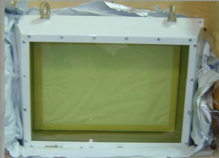
Lead Glass Window for Hot Cell
