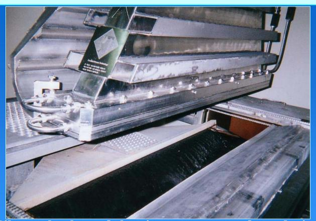
Pilot-scale plant of cleaning waste water from dyeing factories in Korea (treatment capacity 1,000m<sup>3</sup>/day EBM:1MeV, 40kW) Demonstration Plant of 10,000m<sup>3</sup>/day is under construction IAEA Scientific Forum, 27 September 2005
