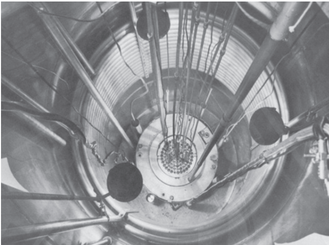
FIG. 3. Original 10 kW TRIGA Mark I core (courtesy of General Atomics).
