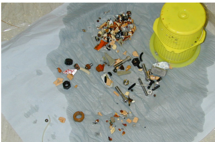
FIG. 32. Collected pieces in the coarse filter (courtesy of Atominstytut, Vienna).
