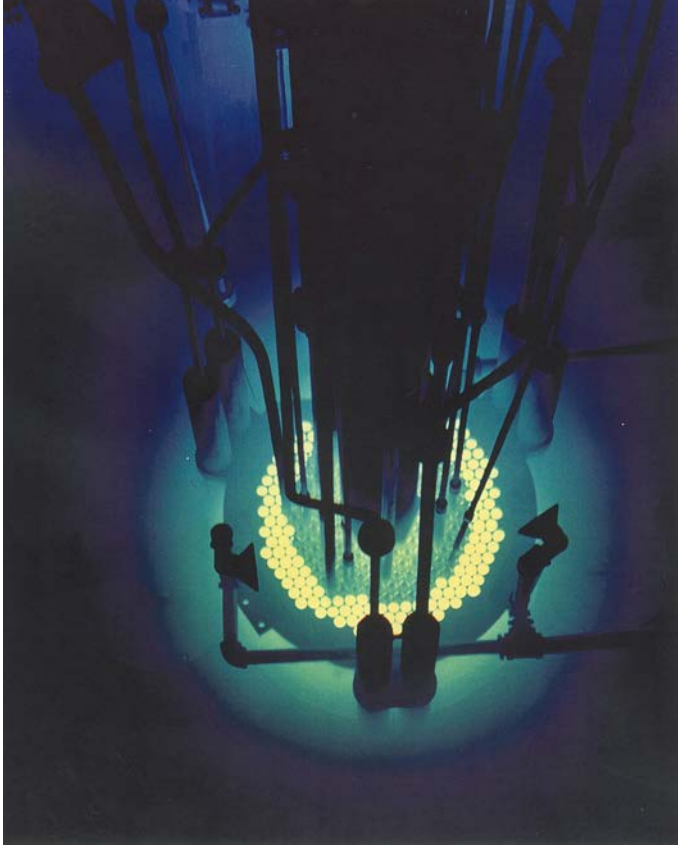
FIG. 20. The TRIGA ACPR core at Tokai Mura, Japan, showing the dry central irradiation cavity (courtesy of General Atomics).
