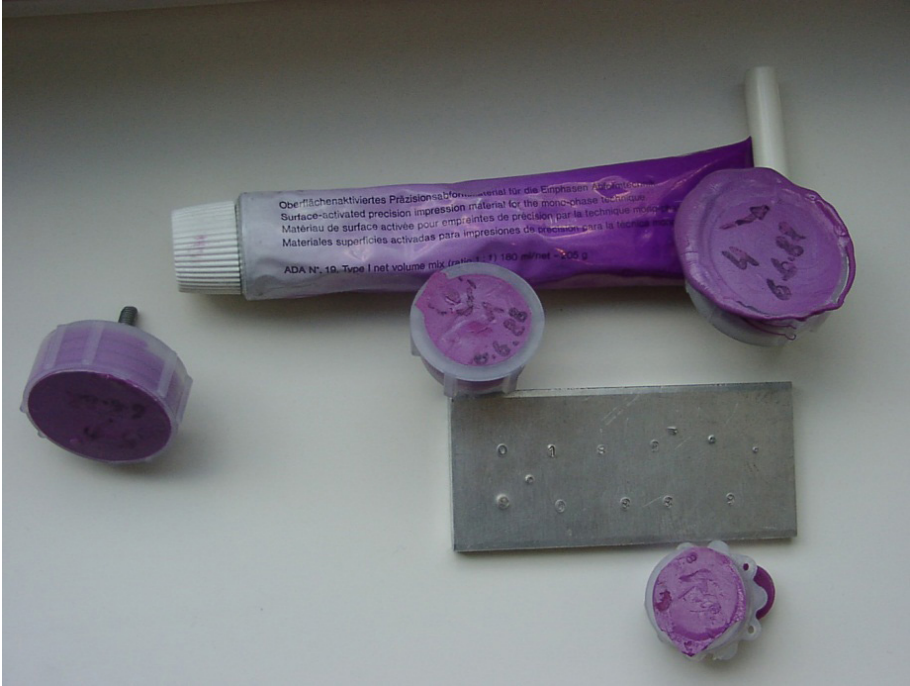
FIG. 36. Replica material to determine the dimension of a corrosion spot (courtesy of Atominstitut, Vienna).
