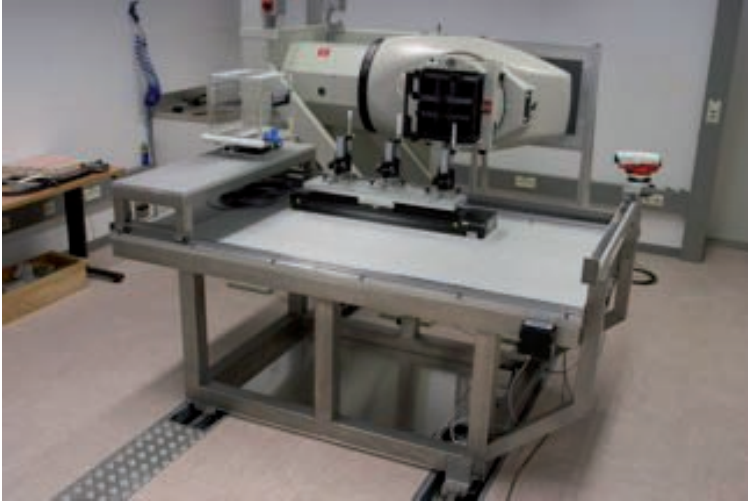
FIG. 4. Measuring bench at the IAEA Dosimetry Laboratory showing a holder for three ionization chambers, mounted on a translation stage, for measurements in air (centre), a water phantom on an elevated rigid frame (left) and a fine focus alignment device (right). The measuring bench can be moved in the beam direction along supporting rails.
