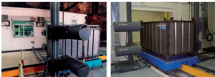
FIG. I-5.2. Box-counter equipment — measuring process.
