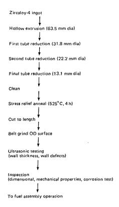
FIG. 36. Production of Zircaloy fuel cladding (typical).
