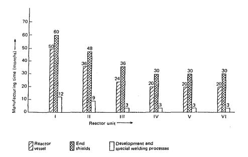
FIG. 12. Manufacturing cycle time of nuclear reactor components.
