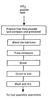
FIG. 35. Basic UO<sub>2</sub> pellet fabrication process.
