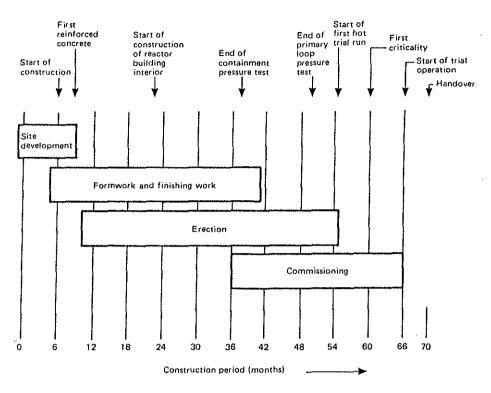
FIG. 25. Construction phases and milestones.
