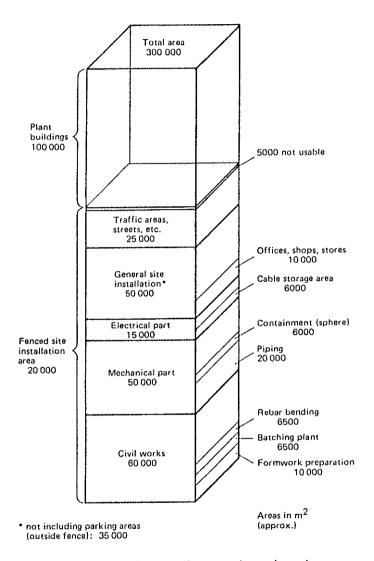
FIG. 31. Areas during civil construction and erection.
