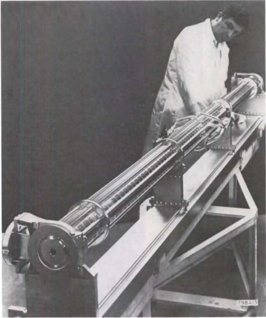
*FIG.1. A ten-foot ( $\approx 3.0$  m) travelling-wave accelerator section for SLAC. With a 16-MW klystron (peak RF power), the energy added by such a section is 40 MeV. The uniform partitioning into RF cavities by annular disks is easily seen. (Reproduced with kind permission of the Stanford Linear Accelerator Center and the Energy Research and Development Administration.)*
