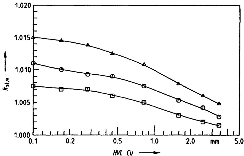
Fig.9. The energy dependence of the factor  $k_{st,w}$  describing the influence of the stem in the water phantom was measured in different phantom materials (squares: SR6, circles: PMMA, triangles: graphite) for the PTW M23331 ionization chamber [29]. The measured values fall on a smooth curve indicating a small measurement uncertainty of about 0.2%.
