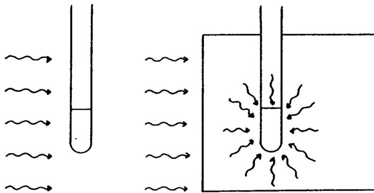
Fig.4. At the calibration of the ionization chamber in terms of air kerma free in air the chamber is exposed to an unidirectional radiation field of a given radiation quality. During the measurement at the depth in the water phantom the radiation field is modified with respect to its spectral and angular distribution.
