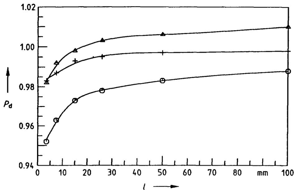
Figs. 8(a) and 8(b). Variation of the displacement correction factor  $p_d$  with the outer diameter for an ionization chamber of 26 mm length (a) and (b) with the length for an ionization chamber with an outer diameter of 7.4 mm, respectively. The radiation qualities correspond to 0.1 mm Cu HVL (circles), 1.23 mm Cu (crosses) and 5.1 mm Cu (triangles). The curves are derived from the work of Ma and Nahum [26].
