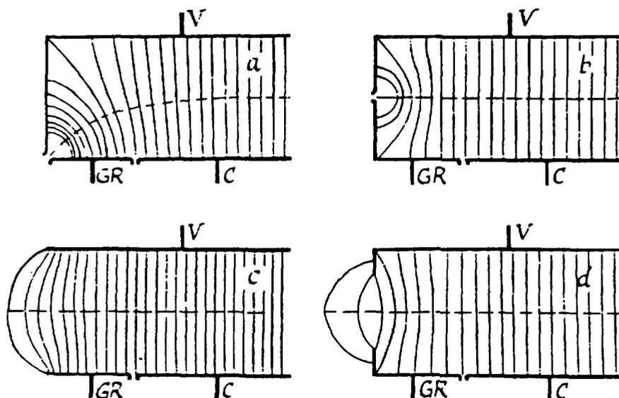
FIGURE 3. Electric field patterns near the edge of a plane-parallel chamber for various guard ring (GR) configurations; charge-collecting electrode denoted by C. (from [1]).
