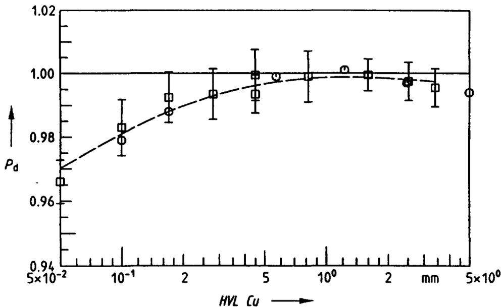
Fig. 7. The component correction factor  $p_d$  for the displacement of phantom material by the ionization chamber. Two Monte Carlo calculations (circles: Ma and Nahum [26]; squares: Seuntjens et al. [13]) were carried out for the NE 2571 ionization chamber with statistical uncertainties of 0.2% and 0.5%, respectively. The dashed curve is a fit to the results by Seuntjens et al.
