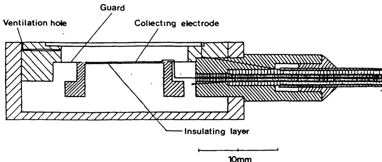
FIGURE 2. The NACP chamber design (from [7]). See text for description.
