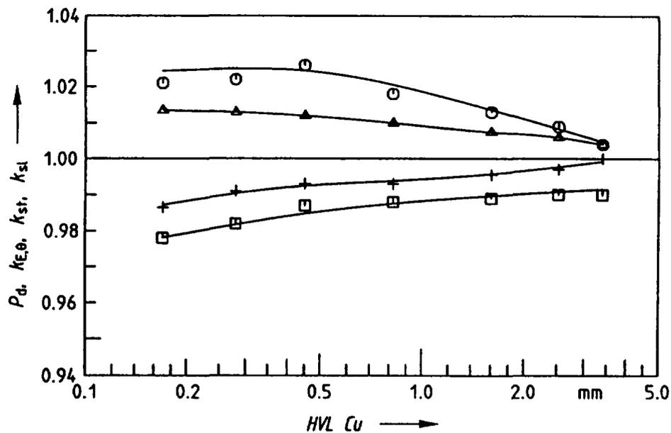
Fig.11. The component correction factor  $p_d$ , (squares)  $k_{E,\theta}$ , (circles)  $k_{st}$  (triangles) and  $k_{sl}$  (crosses) for the PTW M23331 ionization chamber determined by Schneider and Kramer [29].
