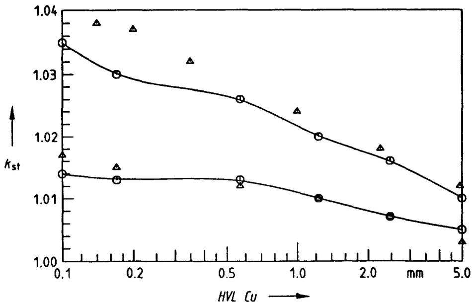
Fig.10. The stem effect correction factor  $k_{st}$  for the NE 2571 (upper curve) and NE 2561 (lower curve) ionization chamber calculated by Ma and Nahum [30] agree very well with measured values for the NE 2561 ionization chamber from Rosser [6] and for the NE 2571 ionization chamber determined experimentally by Seutjens et al. [13]. The maximum difference in the  $k_{st}$  values amount to roughly 2% at low energies.
