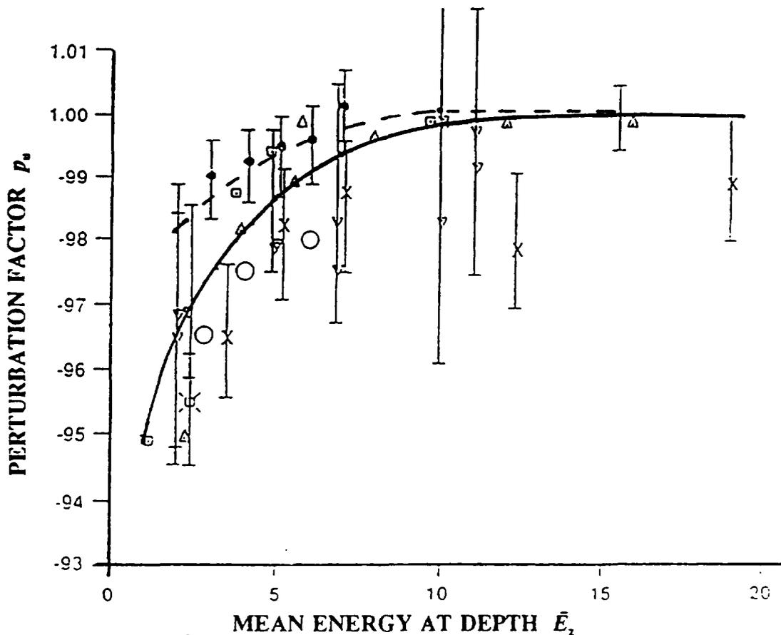
FIGURE 4. Experimental determinations of the perturbation factor  $p_u$ , at  $d_{max}$ , as a function of  $E_z$  for the PTWIMarkus chamber. Data points:  $\square$  [27];  $\nabla$  [28];  $\times$  [29];  $\circ$  [30];  $\bullet$  [9];  $\Delta$  [31]. The full curve is the least-squares fit to the data in [26]:  $p_u = 1 - 0.072 \exp(-.336\bar{E}_z)$ , and the dashed curve is the adopted in [14] (adapted from [26]).
