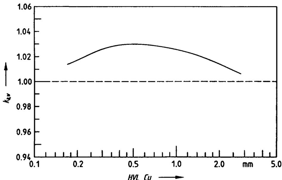
Fig.3. Correction factor  $k_{a,w}$  for the PTW 23331 ionization chamber dependent on the radiation quality characterized by the HVL in Cu. The curve results from smoothed data taken from [3].
