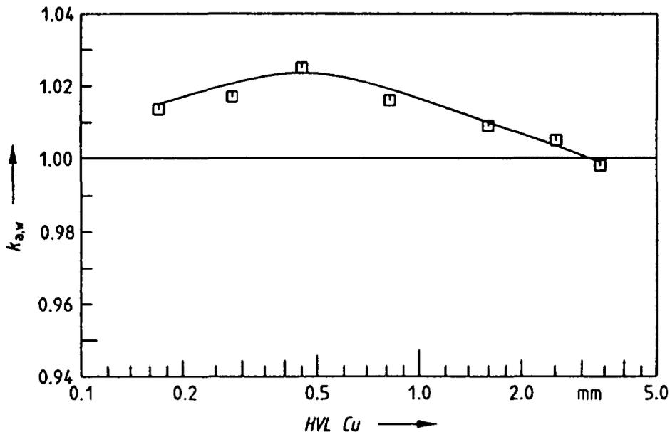
Fig.12. The correction factor  $k_{a,w}$  for the PTW M23331 ionization chamber resulting from the multiplication of the curves given in figure 11.  $k_{sl}$  has not been taken into account, as the sleeve normally used with this chamber will have a much smaller wall thickness than that for which the curve in figure 11 is valid.
