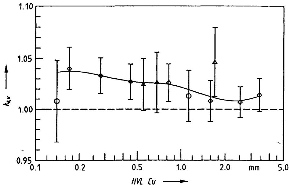
Fig.2. Energy dependence of the correction factor  $k_{a,w}$  derived from the comparison of water absorbed dose calorimetry and air kerma measurement with a Farmer-type ionization chamber. The squares indicate the results of Seuntjens et al., the circles those of Mattsson and the triangles the results from the work of Kubo. The solid curve represents a smoothed mean from all values averaged according to their uncertainties.
