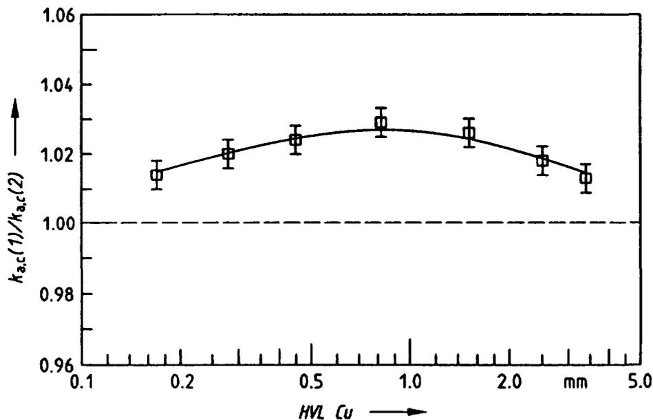
Fig.14. The ratio of  $k_{a,c}(1)/k_{a,c}(2)$  for two different ionization chambers (1:PTW M23331; 2: PTW M23332) as a function of radiation quality.
