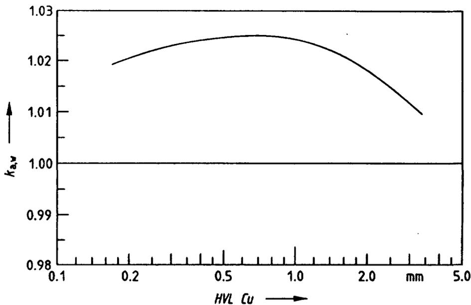
Fig.13. The correction factor  $k_{a,w}$  for the NE 2571 ionization chamber as the product of  $p_d$ ,  $k_{E,0}$ , and  $k_u$  from figures 5,7, and 10 respectively.
