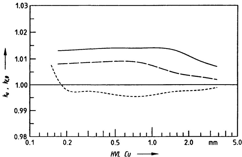
Fig.5. The component correction factor  $k_{E,\theta}$  for the energy and angular dependence of response is shown for two ionization chamber types. For the NE 2571 (solid line) the curve is taken from Seuntjens *et al.* [13] and for the PTW M23331 the reference is Schneider and Kramer [29]. Seuntjens *et al.*, have calculated  $k_u$  for the NE 2571 (dotted line) where only the change in radiation quality between the calibration situation and the in-phantom measurement is taken into account.
