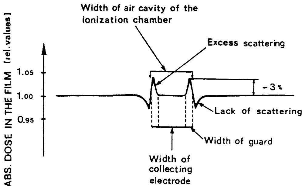
FIGURE 1. *Film measurements across the front surface of a cavity in a PMMA phantom at the depth of maximum dose in an  $E_0 = 6$  MeV electron beam; the effect of the guard ring in reducing the perturbation is clearly demonstrated (from [8]).*
