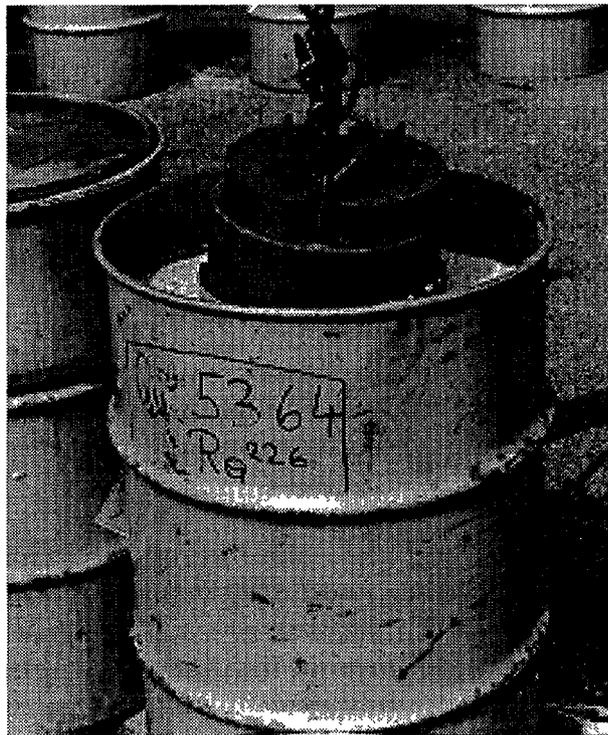
*FIG. A-8. Placing of the lead container in the prefabricated drum.*
