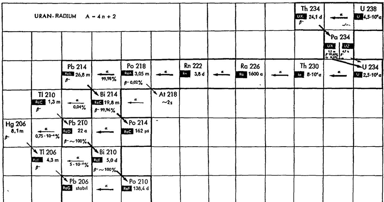
FIG. 2. A simplified scheme for the  $^{238}\text{U}$  decay series, which includes  $^{226}\text{Ra}$ .
