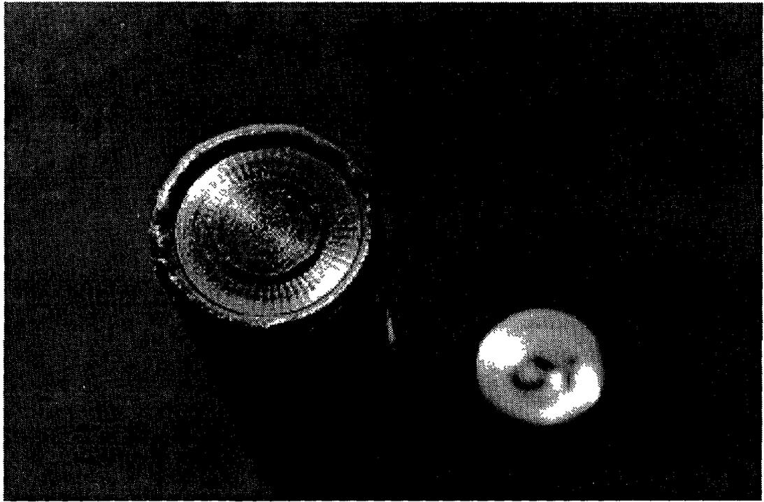
*FIG. A-3. Welded stainless steel capsule.*
