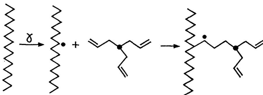
FIGURE 1 Reaction mechanism of multifunctional acrylate with polymer radical by gamma radiation
