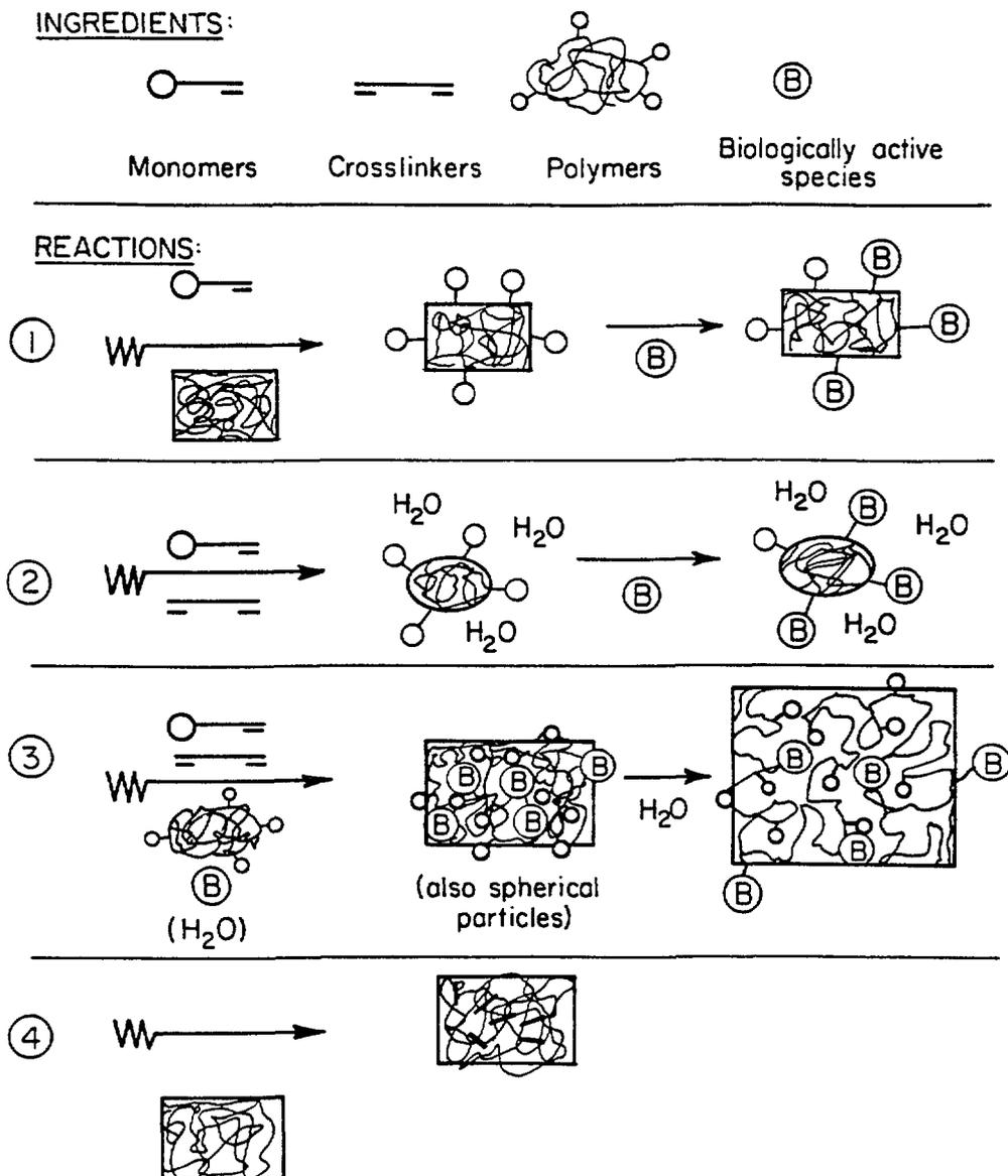
**Fig.2. Radiation processes for producing new or modified polymeric biomaterials. Note that biomolecules (B) are chemically attached after processing or physically entrapped during processing (2)**
