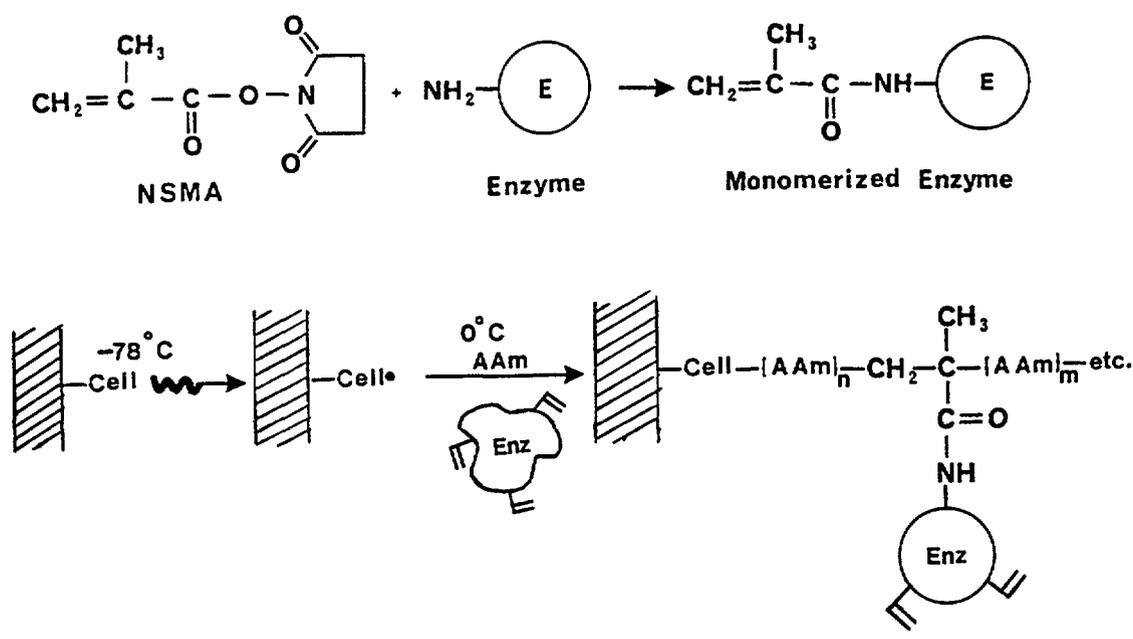
**Fig.4. New radiation graft method for immobilizing a monomer-conjugated biomolecule as an enzyme (13)**
