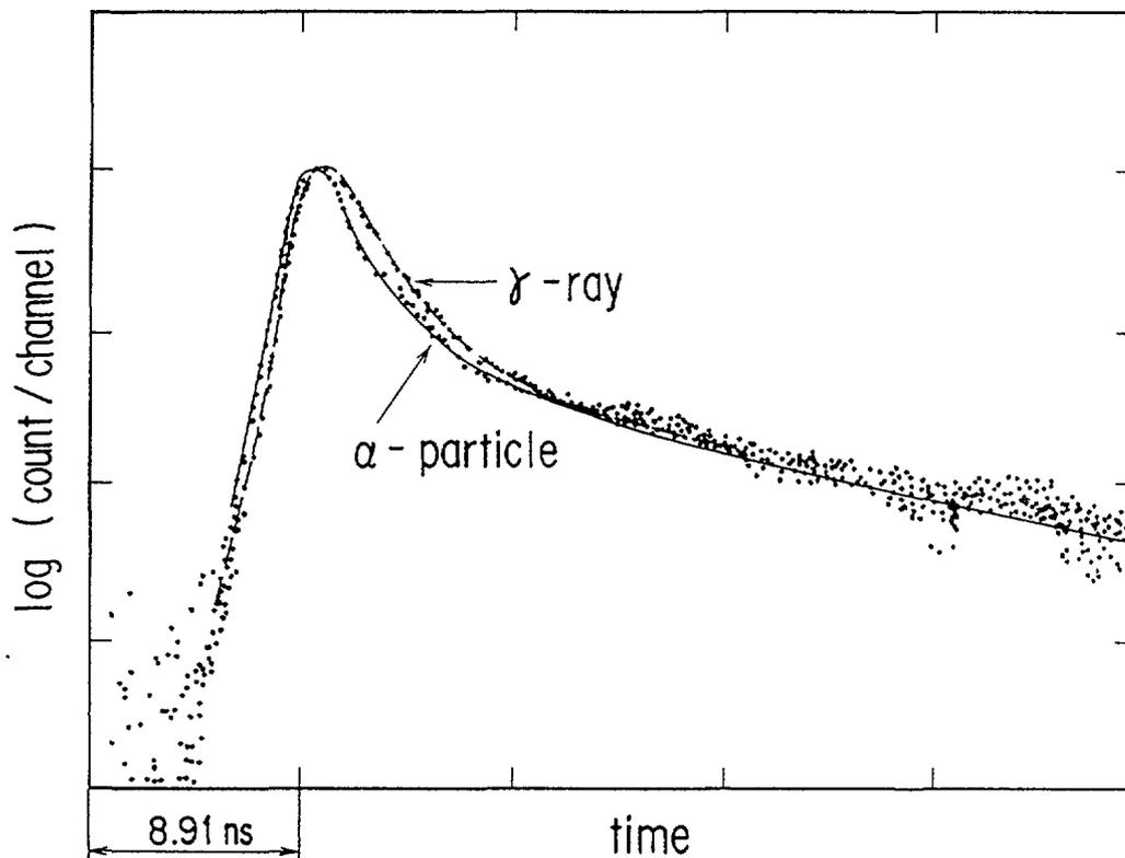
Fig. 4 Decay of PPO Singlet State in Cyclohexane
