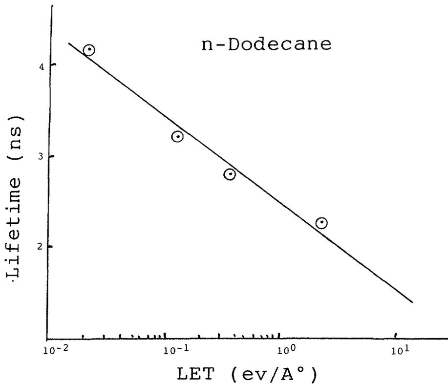
Fig. 3 L.E.T. Dependence of Lifetime of Singlet Excited State
