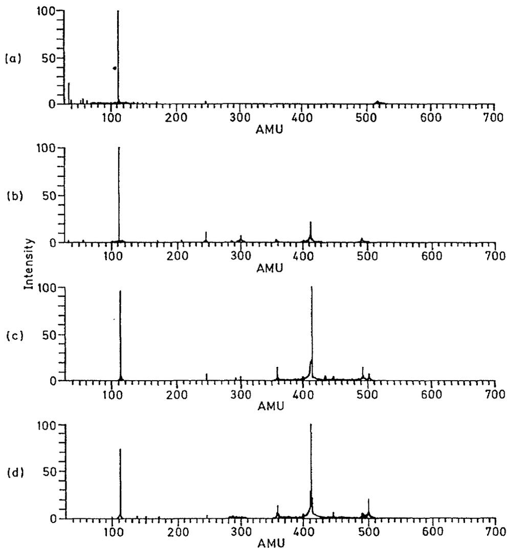
FIGURE 2 FTICR spectra for TPGDA (molecular ion m/z 300) (a) EI, (b) CI 2sec, (c) CI 20sec, (d) CI 60sec.
