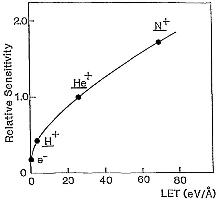
Fig. 6 Relative Sensitivity of Crosslinking in Polystyrene by Various Ion Beams (Normalized at 1MeV  $He^+$  Ion)
