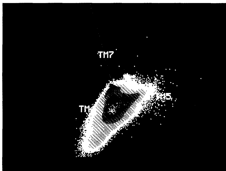
FIG. 7.17. Landsat TM (4-5-7) feature space with the training data points in the centre.
