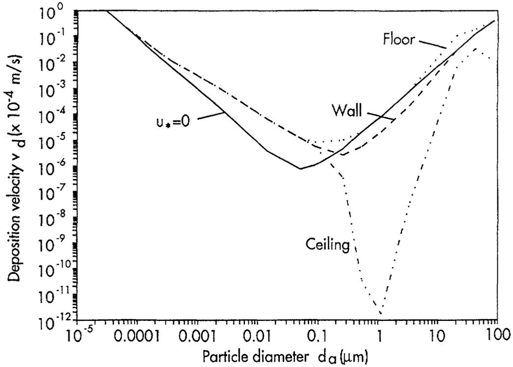
FIG. 6. Comparison of deposition velocity onto smooth surfaces (floor, wall and ceiling) for a friction velocity ( $u_*$ ) of  $3.41 \times 10^2 \text{ m s}^{-1}$  [18].
