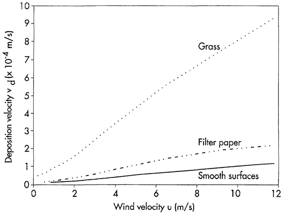
FIG. 3. Deposition velocity for natural radioactive aerosols as a function of wind velocity [8].
