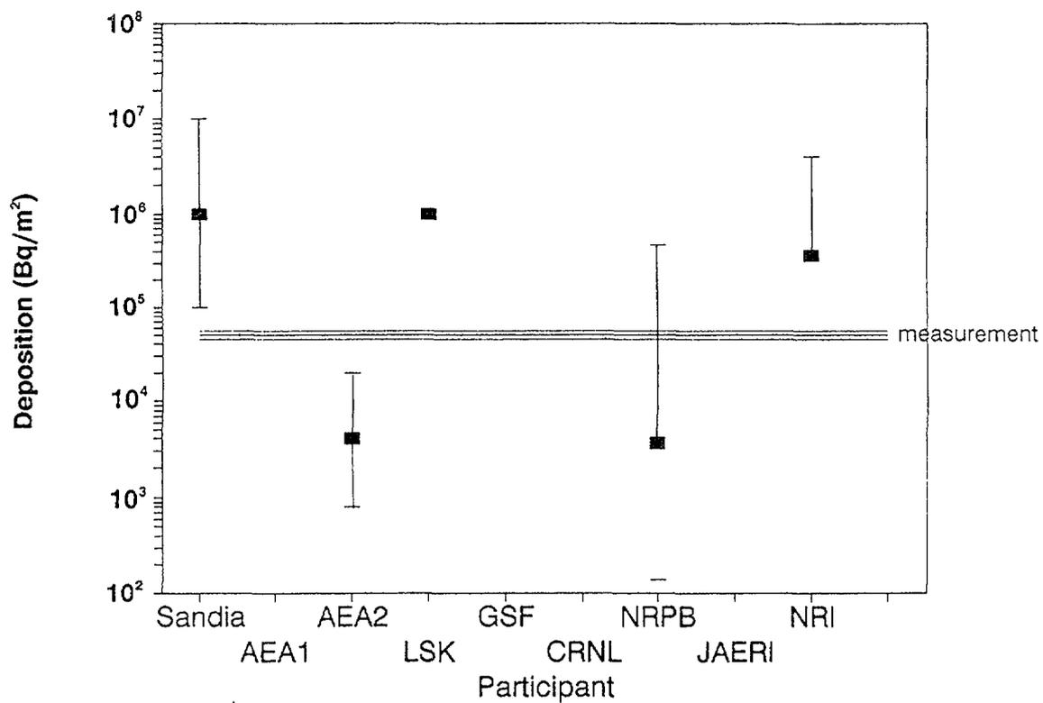
FIG. A-12. Estimates of elemental  $^{131}\text{I}$  dry deposition on internal surfaces.
