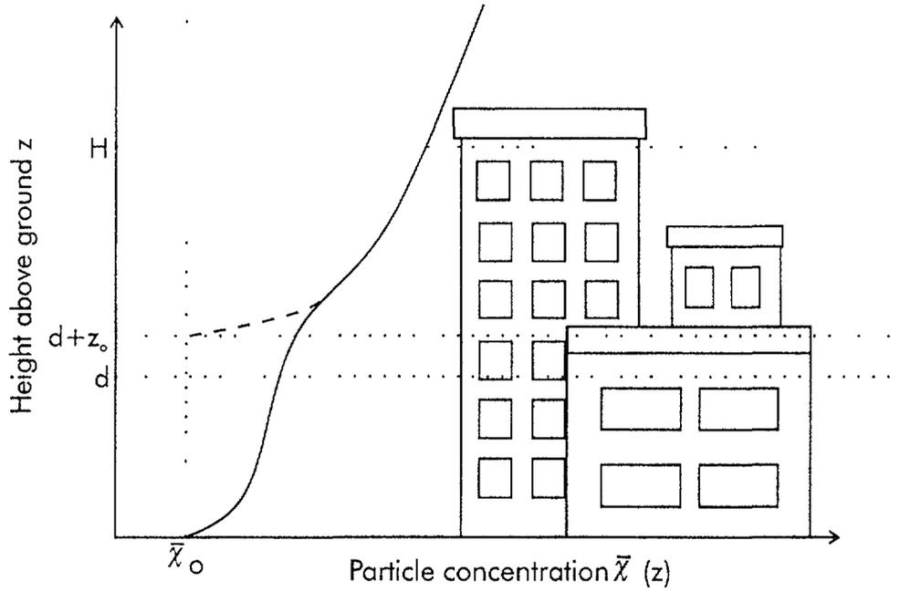
FIG. 2. Mean particle concentration as a function of height above ground.
