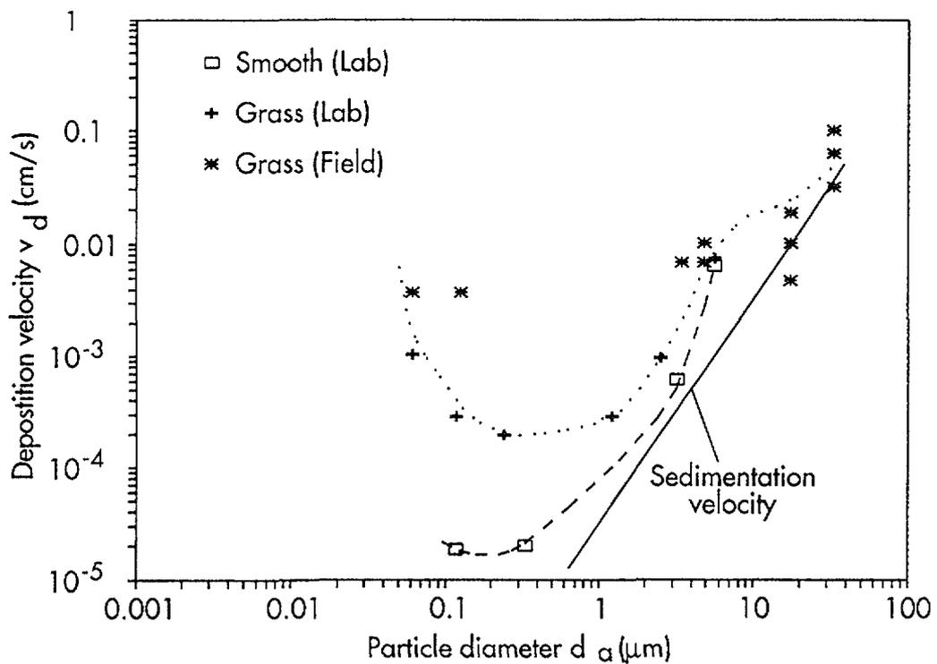
FIG. 4. Deposition velocity to grass and smooth surfaces as a function of particle size [14].
