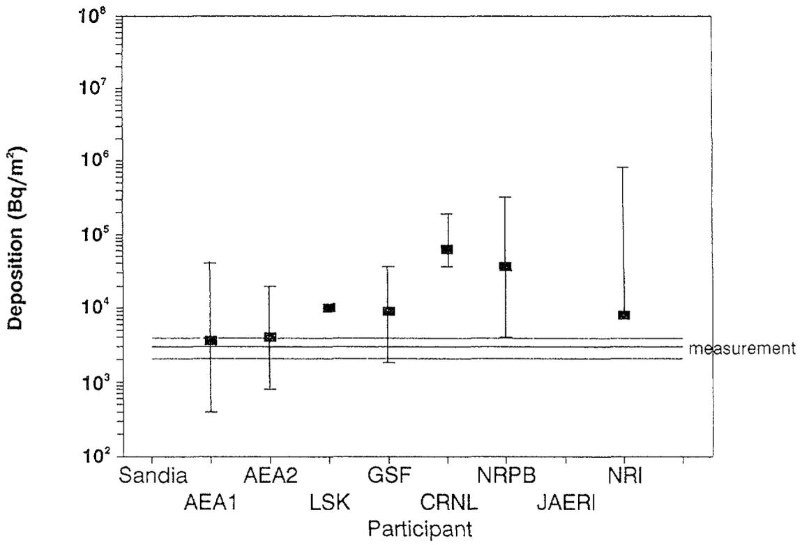
FIG. A-3. Estimates of <sup>137</sup>Cs dry deposition on walls.
