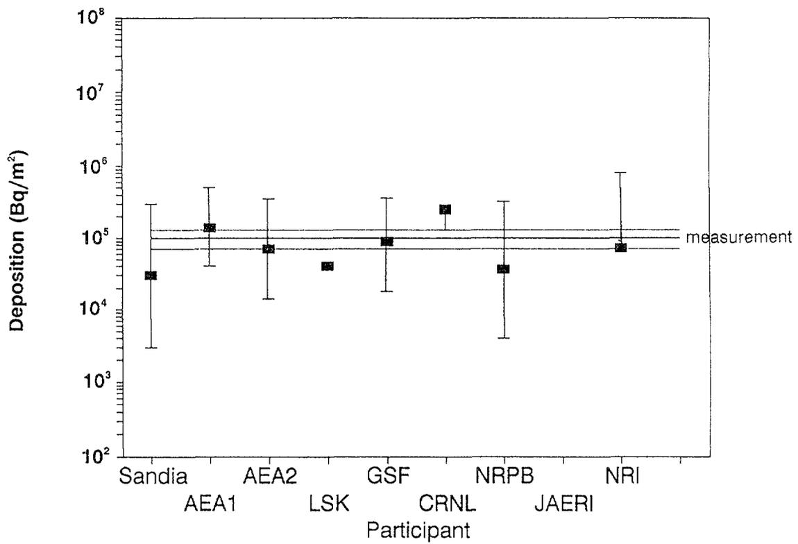
FIG. A-4. Estimates of <sup>137</sup>Cs dry deposition on roofs.
