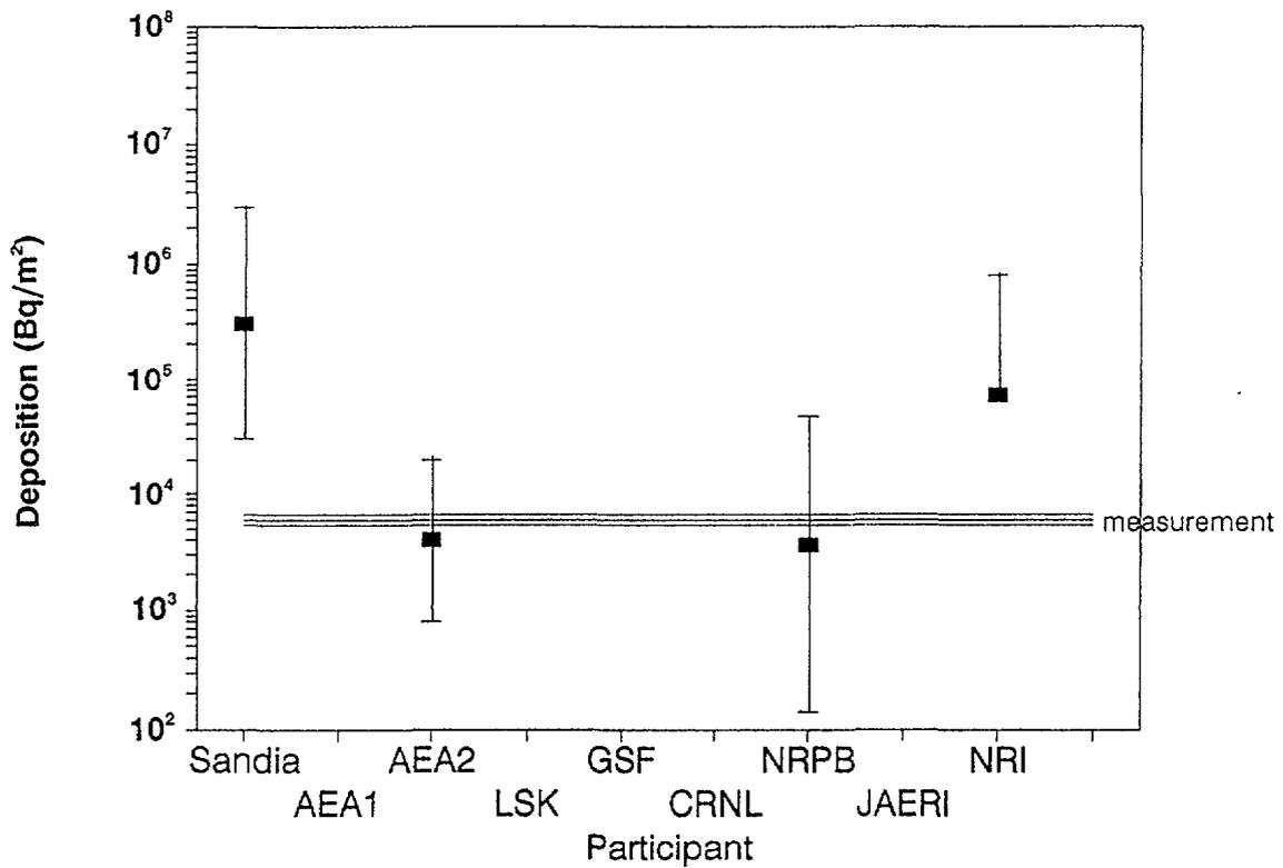
FIG. A-6. Estimates of <sup>137</sup>Cs dry deposition on internal surfaces.
