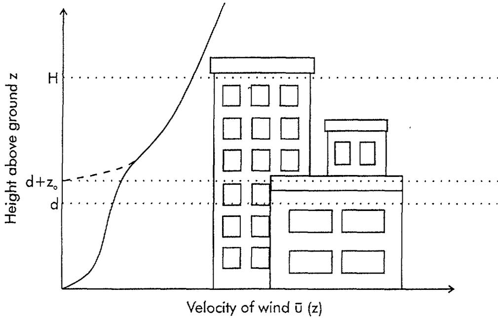
FIG. 1. Mean horizontal wind velocity as a function of height above ground.
