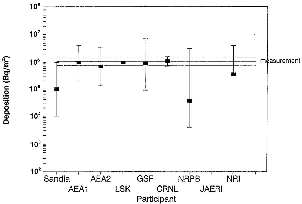
FIG. A-10. Estimates of elemental <sup>131</sup>I dry deposition on roofs.
