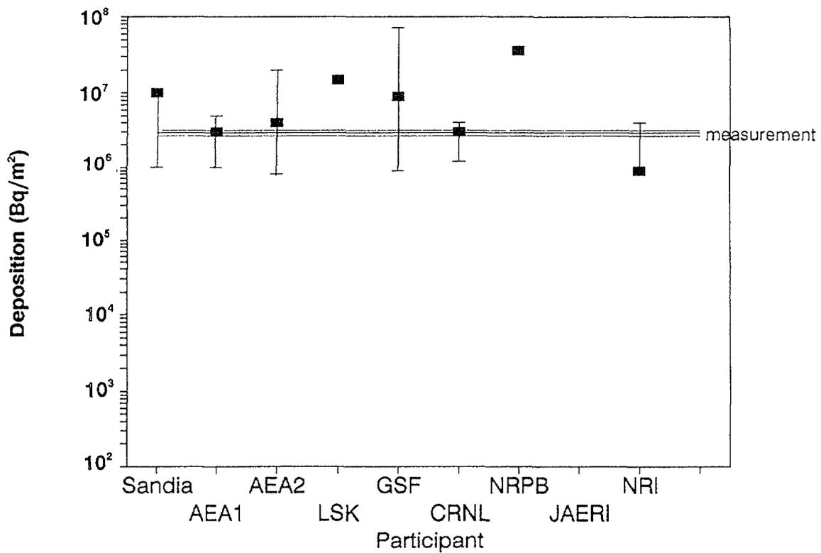
FIG. A-11. Estimates of elemental  $^{131}\text{I}$  dry deposition on trees.
