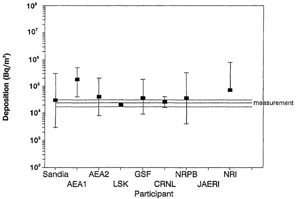
FIG. A-2. Estimates of <sup>137</sup>Cs dry deposition on roads.
