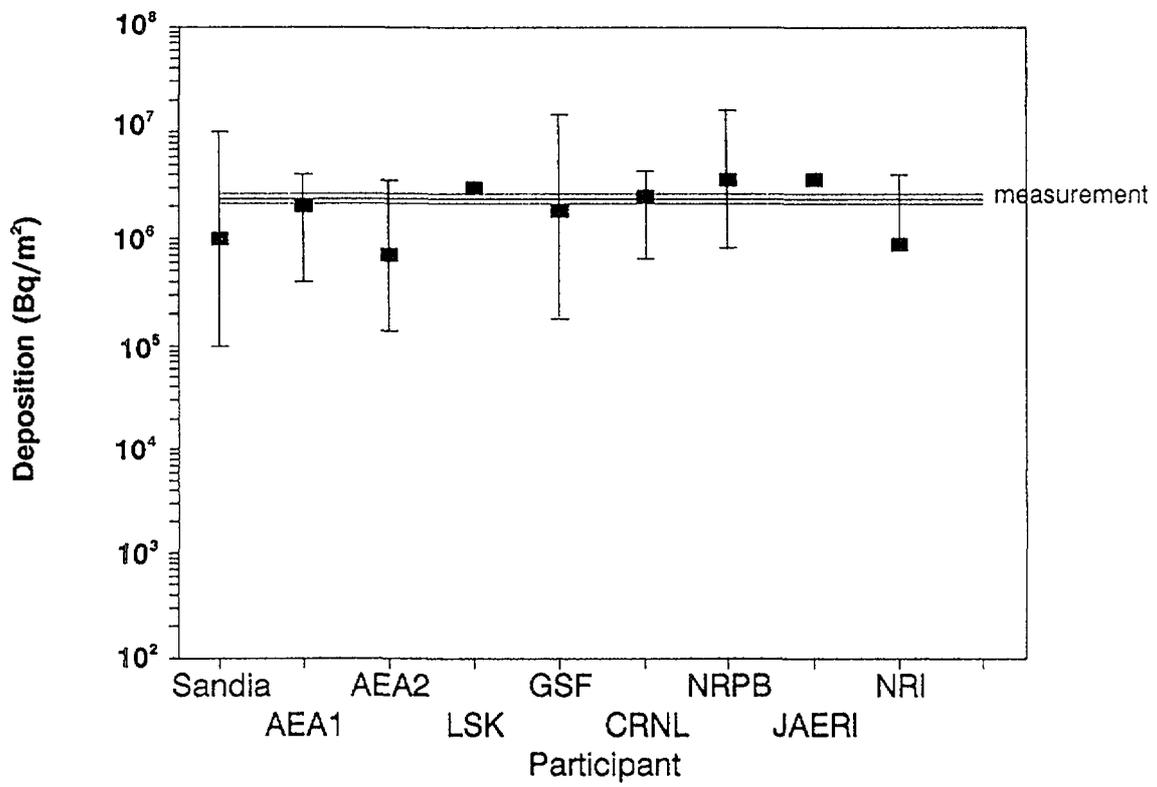
FIG. A-7. Estimates of elemental <sup>131</sup>I dry deposition on grass.
