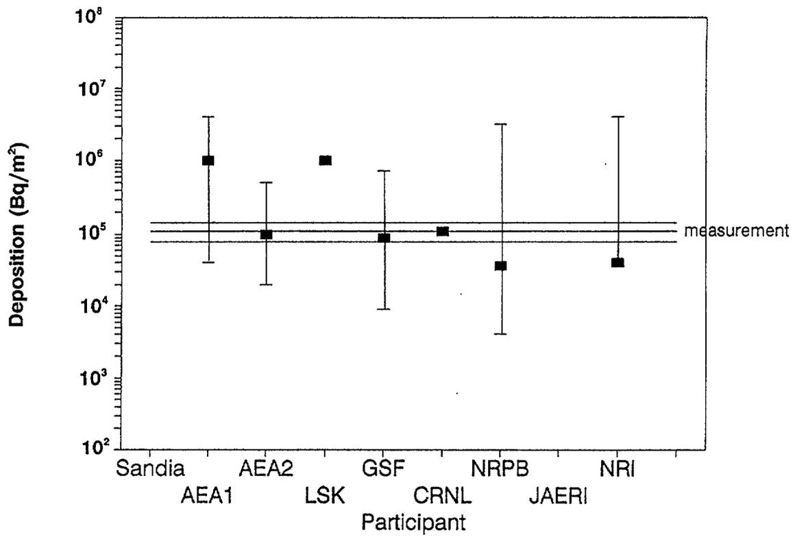
FIG. A-9. Estimates of elemental <sup>131</sup>I dry deposition on walls.
