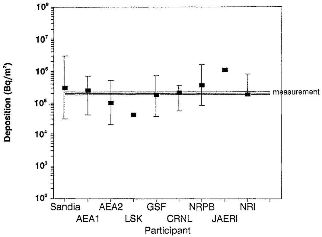
FIG. A-1. Estimates of <sup>137</sup>Cs dry deposition on grass.
