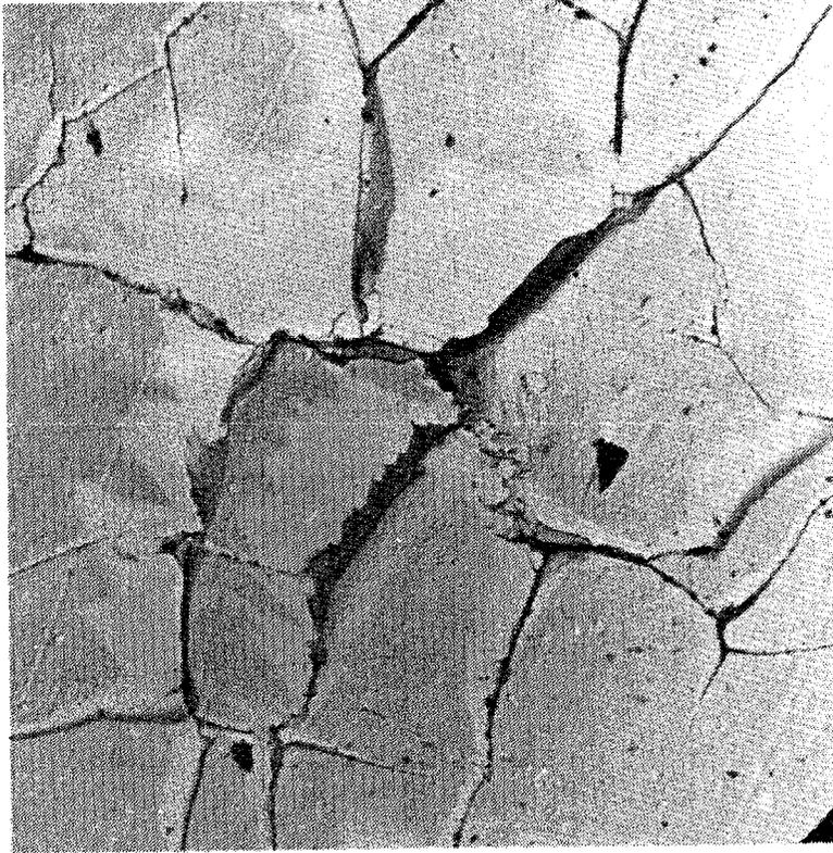
*FIG. 2.22. Zircaloy-2 surface after oxidation in steam at 350°C (billet Z8006, 192 days at 350°C, weight gain 40 mg/dm<sup>2</sup>) (6000×) - specimen surface was uniformly covered with cracks at about this frequency [5].*
