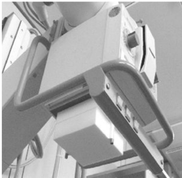
Fig. III-3. Pre-filter attached to X ray Tube assembly.
