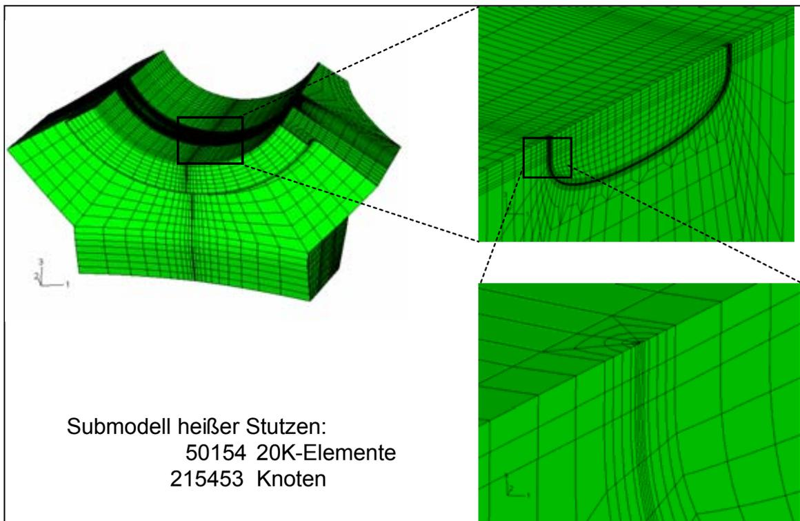
FIG. G14 – Detail of the outlet nozzle corner crack with half elliptical shape in base material.
