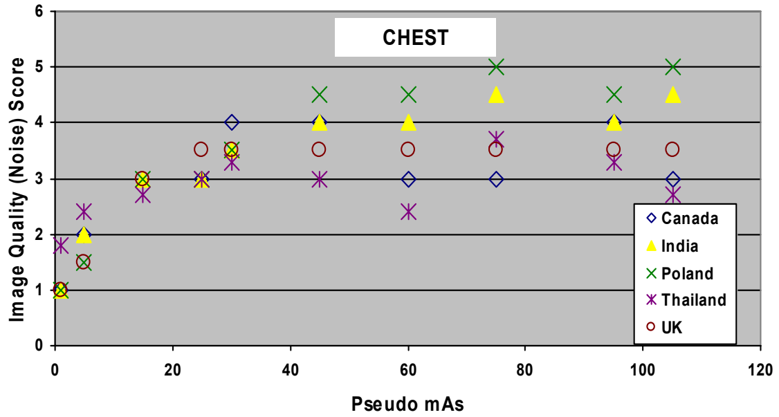
FIG. 2. Image quality scores for chest CT images for radiologists from different countries.
