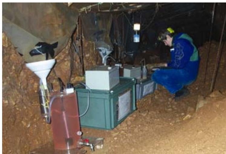
FIG. 5. Construction for collecting water samples in the tunnel with automatic device for flow rate and fluorometer for the multitracer experiment.
