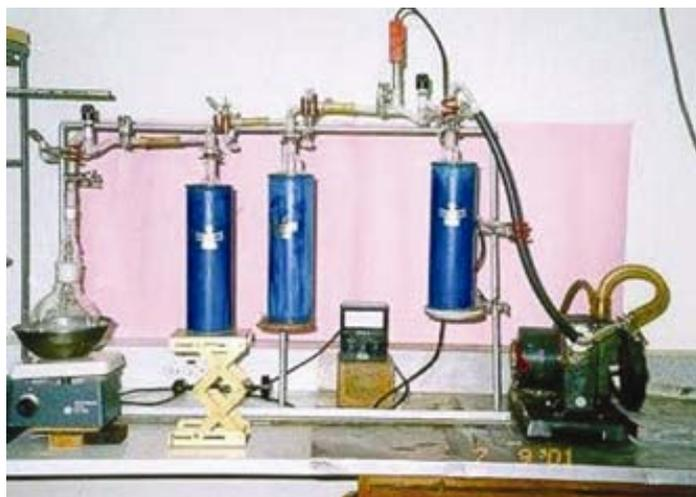
*FIG. 3. Soil moisture extraction system.*
