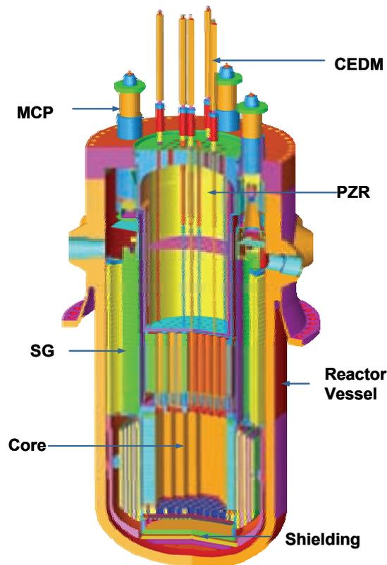
Figure 13. SMART reactor assembly.
