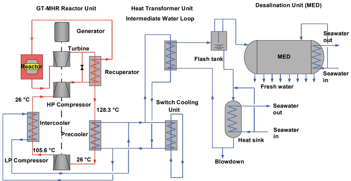
Figure 31. Principle of waste heat utilisation from a GT-MHR (or PBMR).
