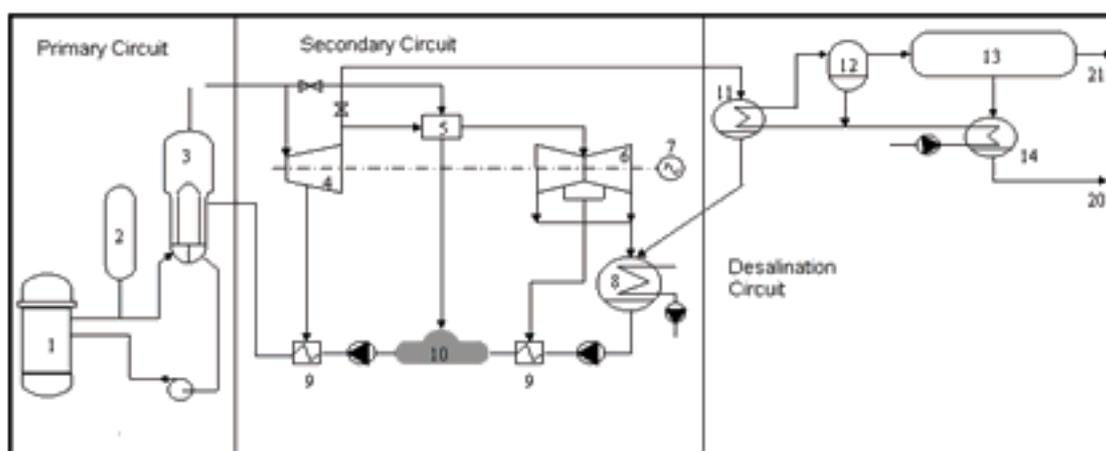
1: Reactor core, 2: Pressurizer; 3: Steam generator; 4: High pressure turbine; 5: Intermediate steam heater; 6: Low-pressure turbine, 7: Generator, 8: Main condenser, 9: Pre-heaters, 10: De-aerator; 11: Seawater heater; 12: Flash tank, 13: MED plant, 14: MED output condenser, 20: Fresh water out, 21: Brine out-fall.
