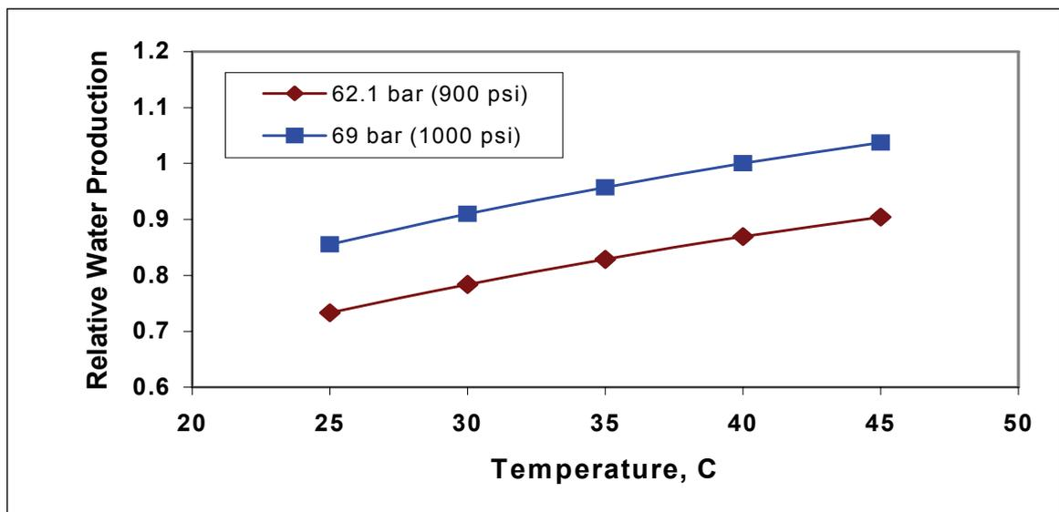
Figure 32. Normalized water production as a function of RO feed water temperature and pressure.
