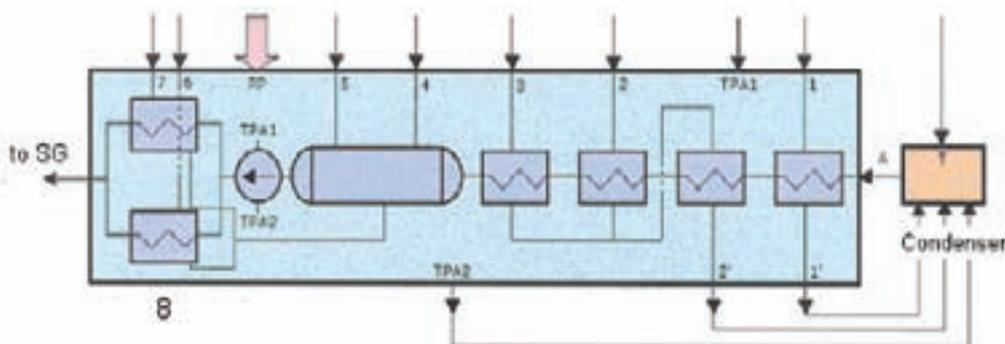
1, 2, 3- LP turbine outputs; 4- Dryer; 5, 6- HP turbine outputs; 7- Super-heater; RP- Condensate return from the desalination plant; 8-Reheater; TPA1-Input to turbine driven feed water pump; TPA2- Output from turbine-driven feed water pump; 1'- Reheater output R1; 2'- Reheater RP output; SG- Input to steam generator.
