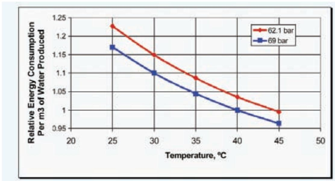
Figure 33. Specific consumption as function of feed temperature and pressure.
