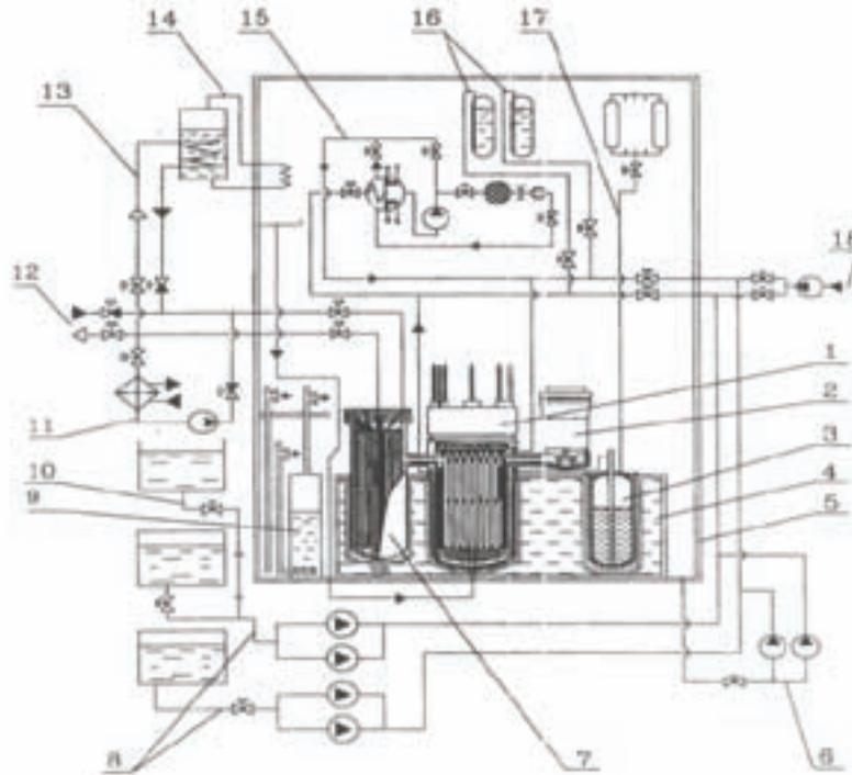
Figure 14. General layout of the KLT-40 reactor.
