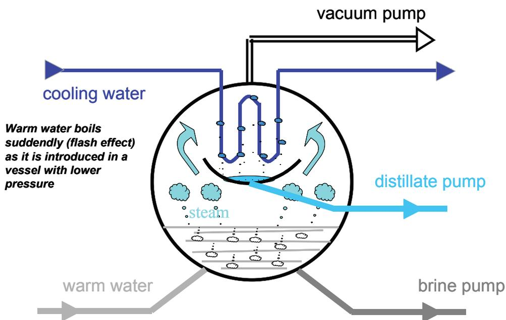
Figure 19. Operating principle of a single stage MSF.
