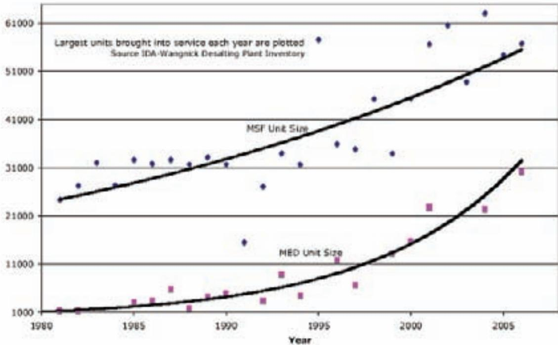
Figure 28. Unit size growth of MSF and MED plants over the years. [8].
