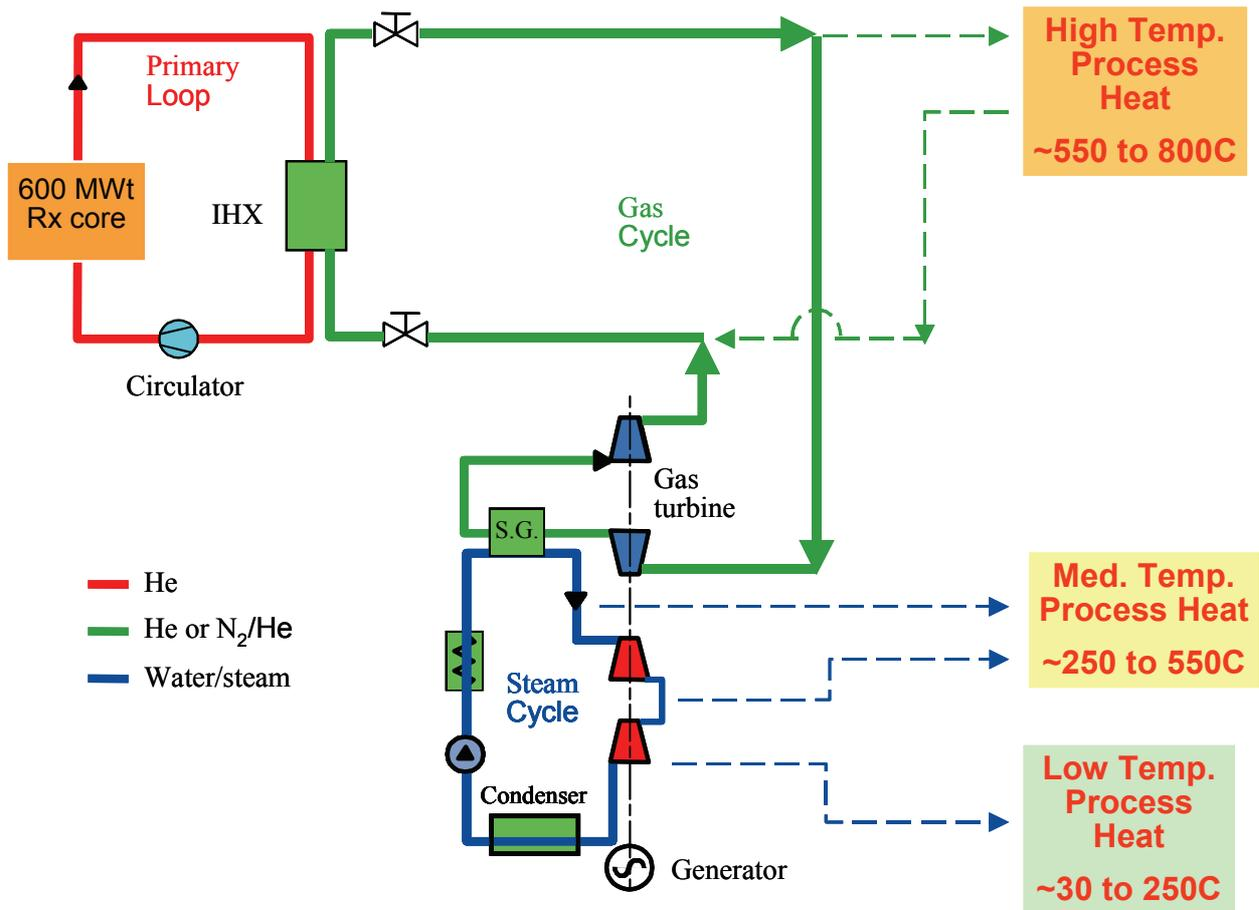
Figure 17. Different uses of ANTARES.
