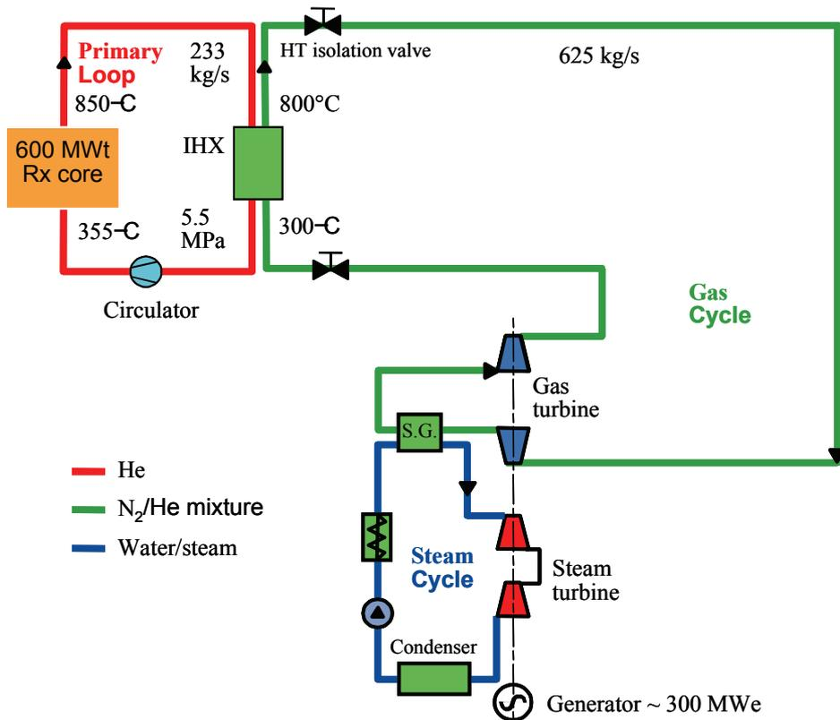
Figure 16. Principle of ANTARES operation with a combined cycle power conversion system.
