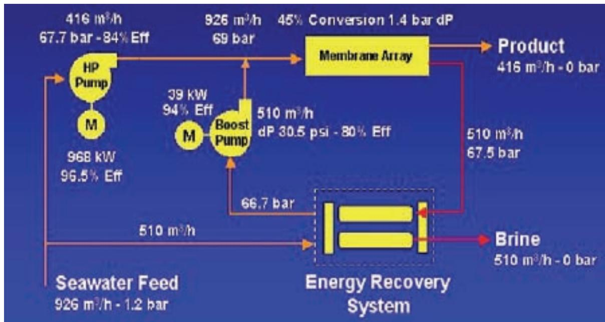
Figure 30. Principle of a RO Work Exchanger [8].
