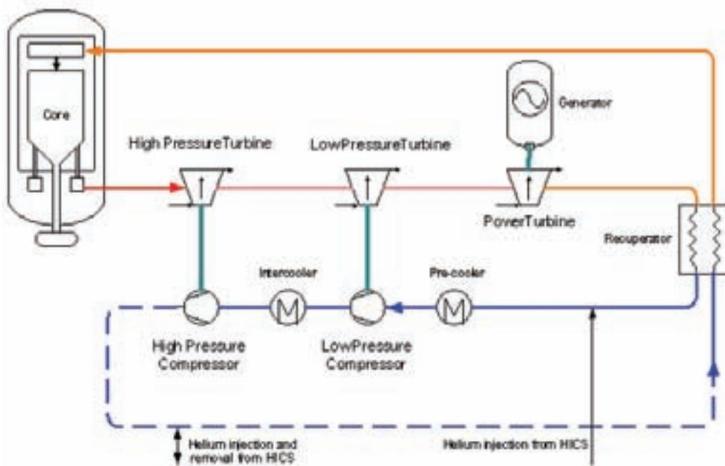
Figure 10. Power conversion system of a PBMR.
