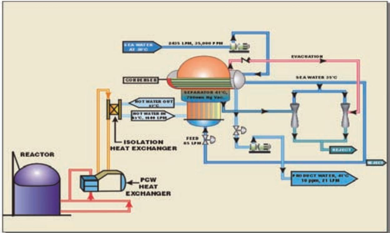
Figure 34. LTE-MED system coupled to CIRUS reactor.
