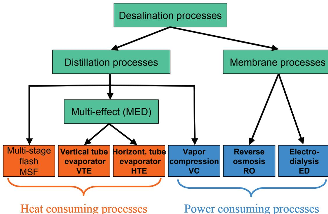
Figure 18. Desalination processes.
