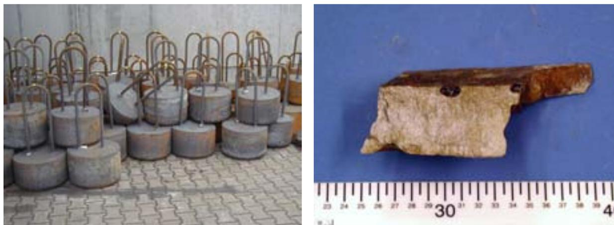
FIG. 3. Ferro-tungsten ingots and details of the metal structure.
