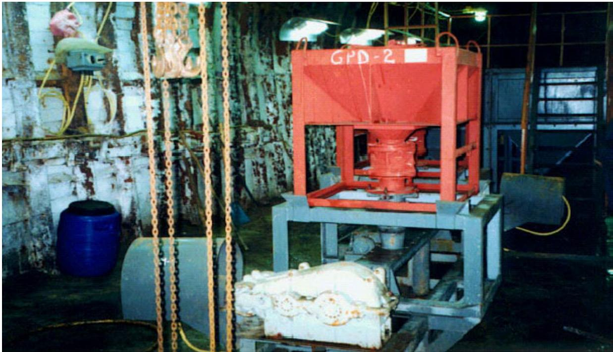
*FIG. 1. Underground treatment station — the feeder of the purification agent.*
