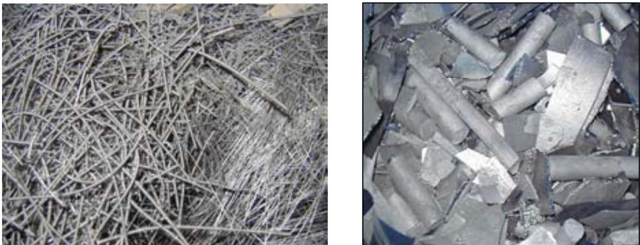
*FIG. 1. Filament and pressed powder residues.*
