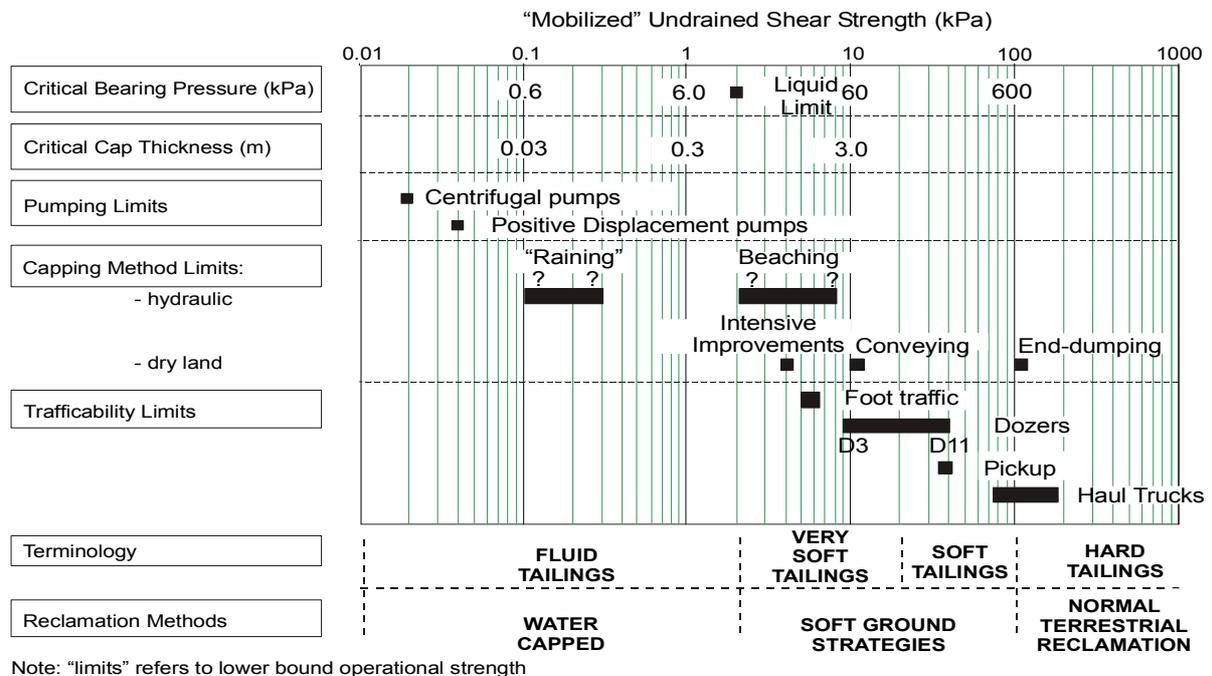
FIG. 4. Remediation methods as a function of tailings shear strength and critical parameters.
