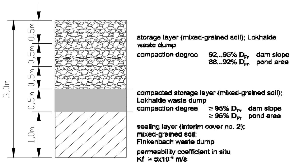
FIG. 5. Layering of the final cover on the northern tailings beaches of Pond A.
