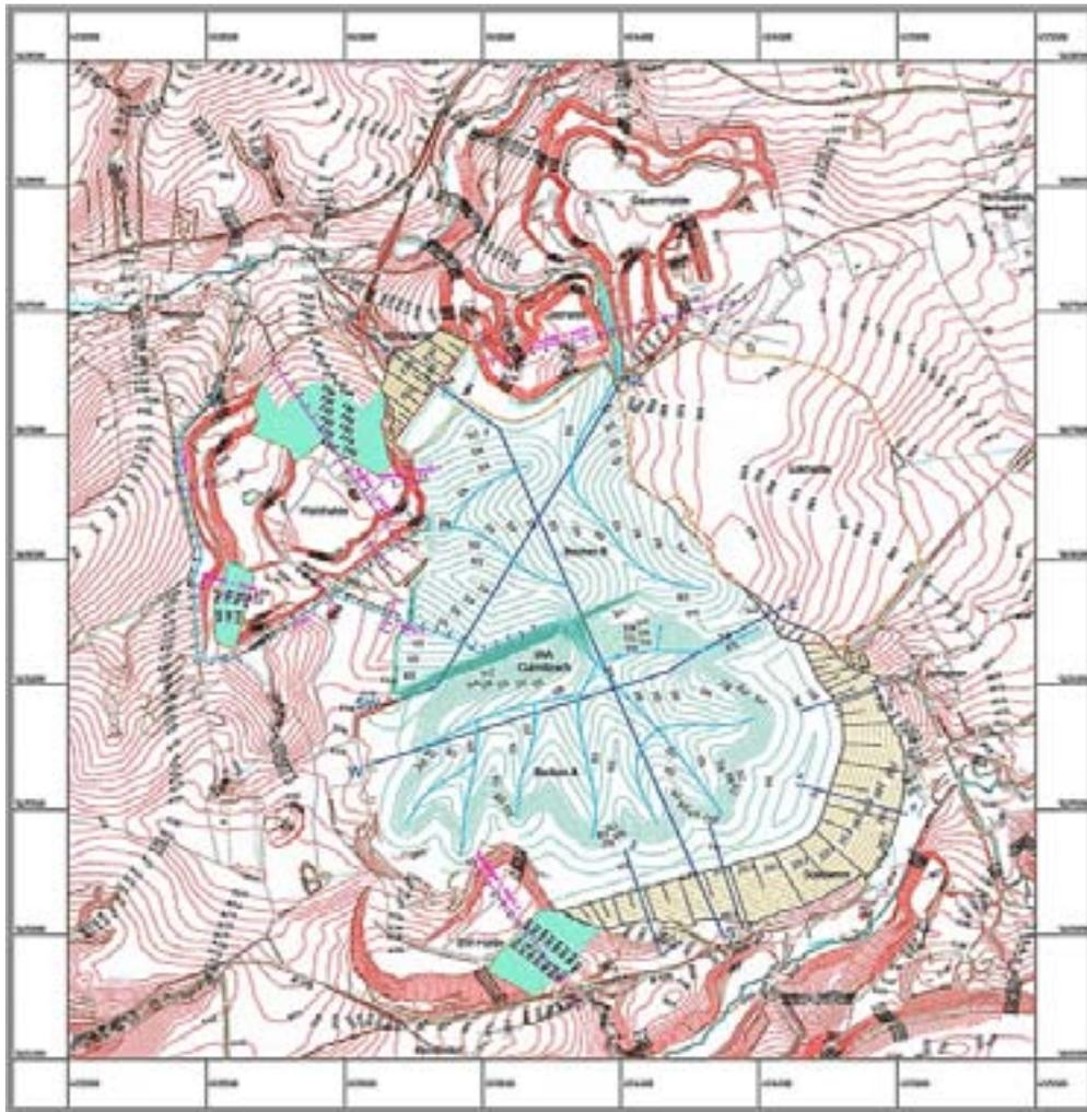
FIG. 3. Conceptual design of the re-contoured Culmitzsch tailings pond.
