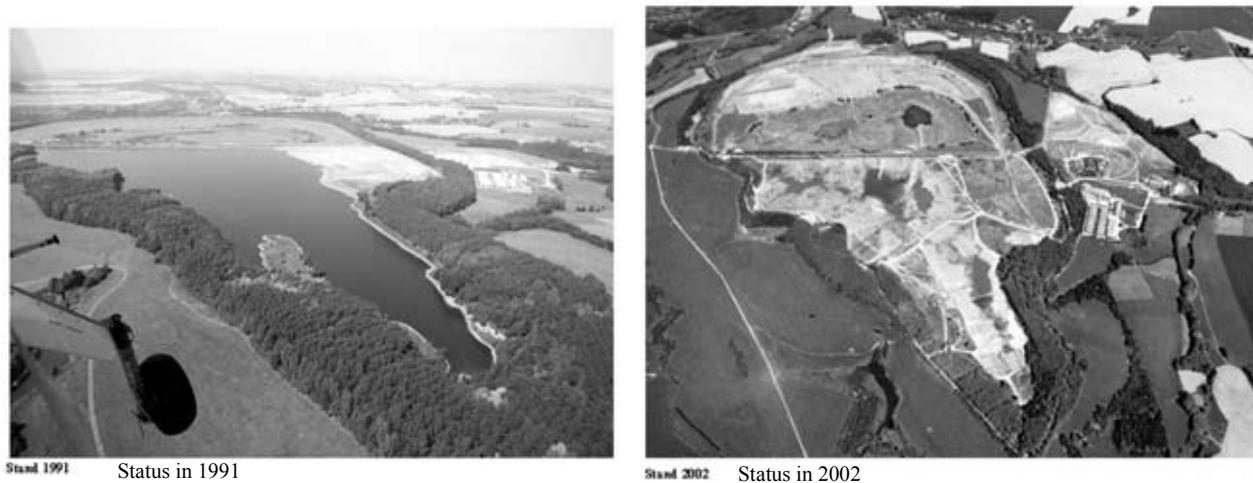
FIG. 5. The Trünzig tailings pond in 1991 and after placement of the interim cover in 2002.
