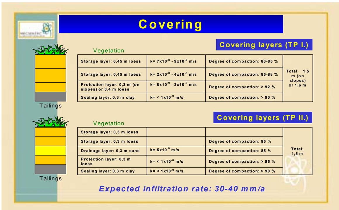
FIG. 4. Structure and composition of the covering.
