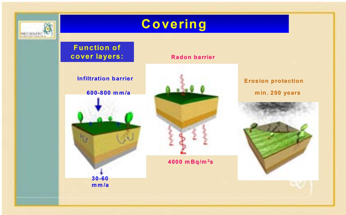
FIG. 3. Function of the covering layer.
