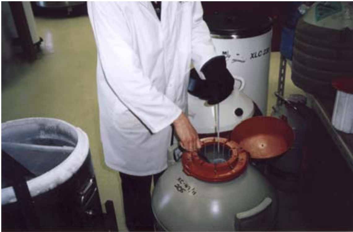
Fig. 10. When transferring frozen straws the canister should not be brought beyond the neck of the container. It should not remain there for more than 10 seconds.
