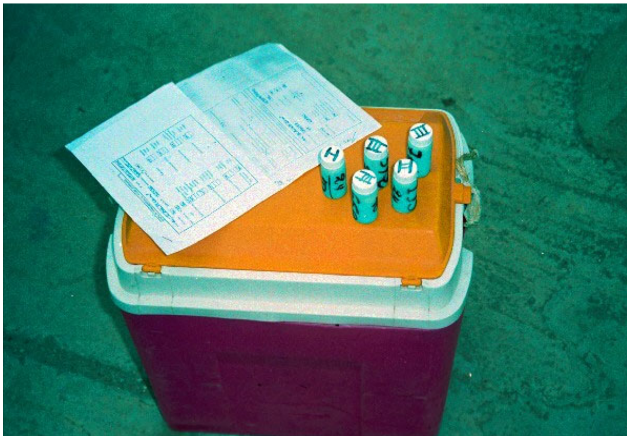
Fig. 12. Milk samples from a herd in Tunisia, preserved with sodium azide, being sent on ice to the laboratory for RIA of progesterone.
