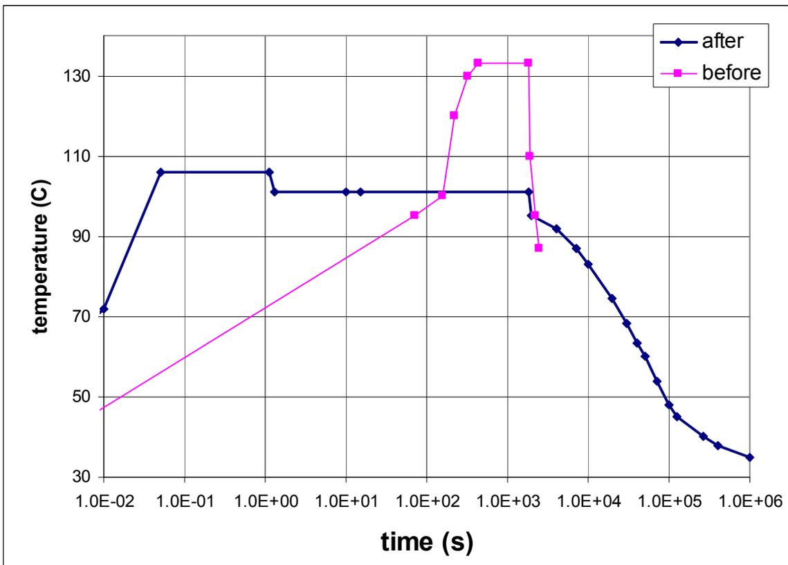
Figure 3 Temperature for Steam Generator Blowdown Break (SGBDB) in IB rooms with potential break locations
