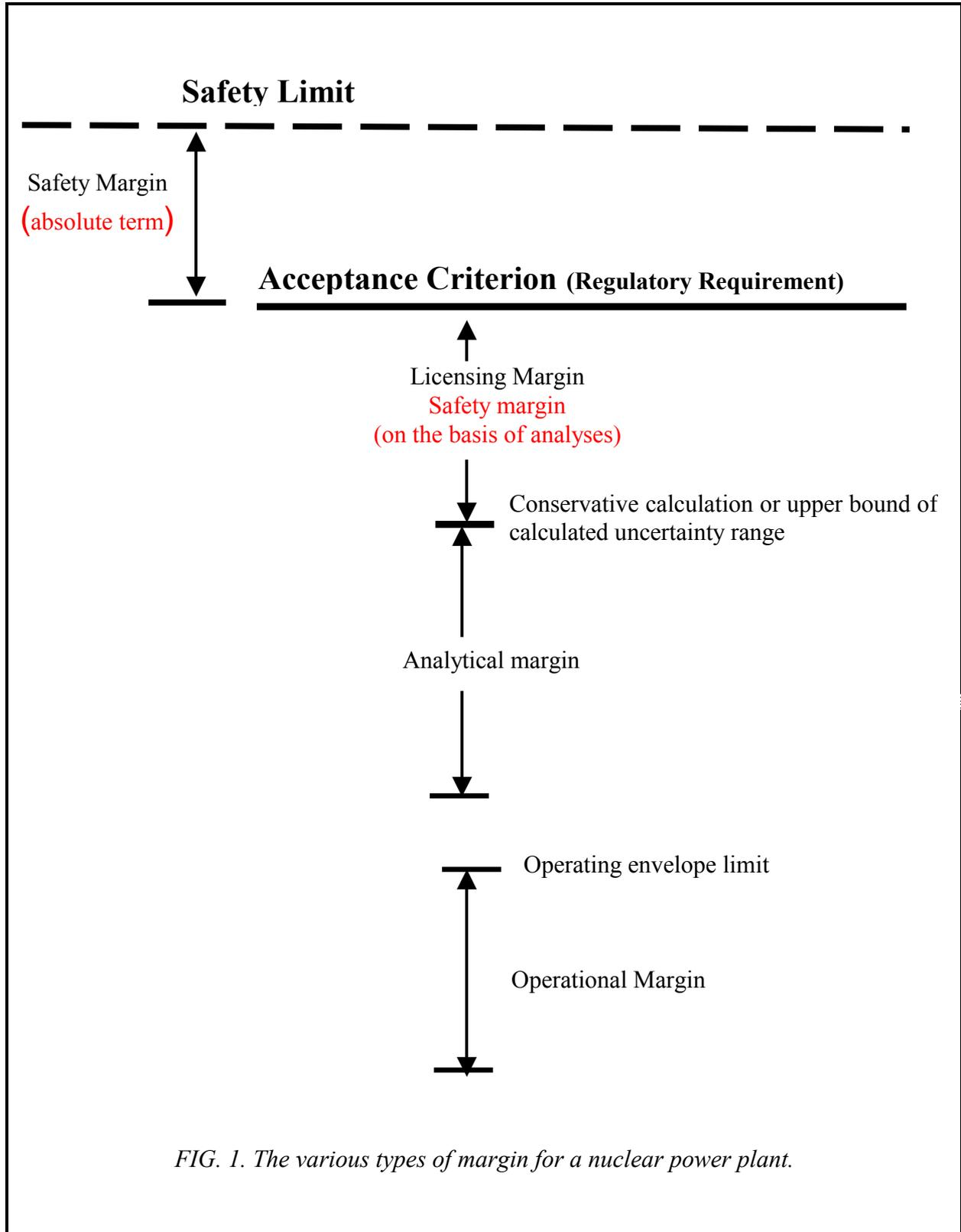
FIG. 1. The various types of margin for a nuclear power plant.
