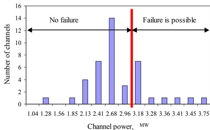
Fig. 8. Real distribution of FC power in the most loaded GDH at 4200 MW power level
