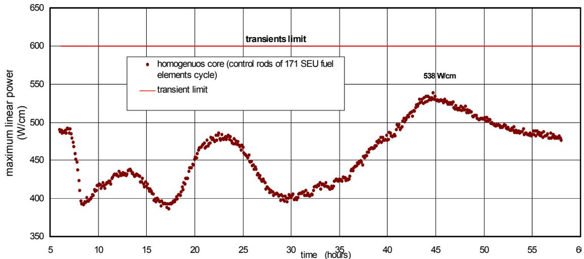
The PCI effect was carefully analysed. In all the cases, the calculations showed that the linear power and its variation during the load cycles were below of allowed limits.
