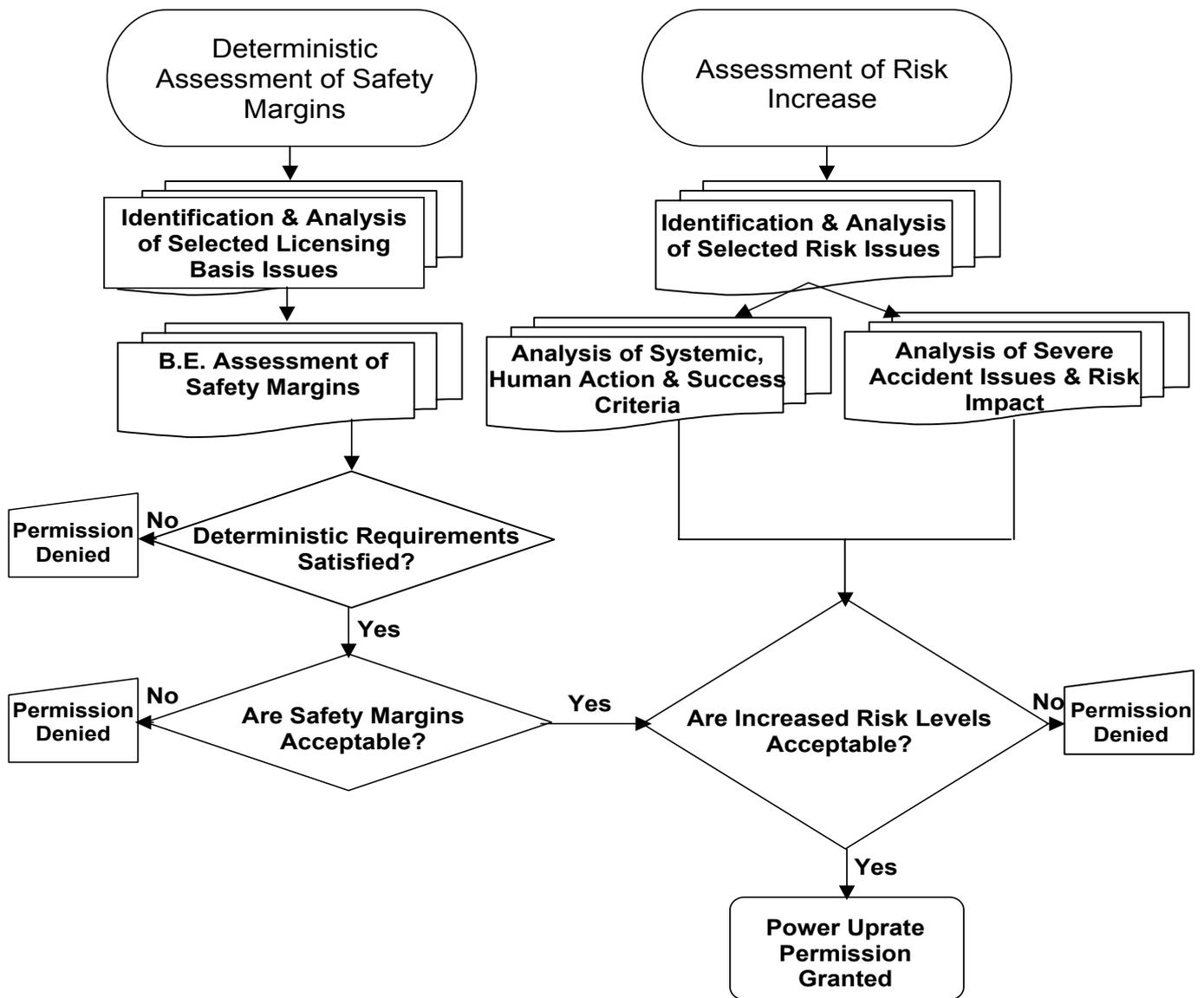
Figure 1 Flow chart depicting regulatory process for plant power uprate assessment
