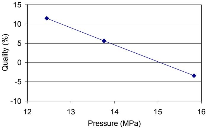
Figure 3 – Critical quality versus pressure for constant heat flux and  $G \cong 1,370 \text{ kg s}^{-1}\text{m}^2$ .
