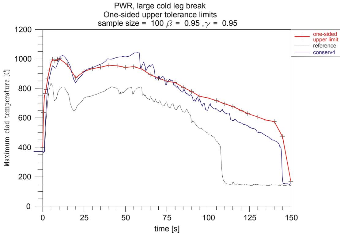
Figure 1: Calculated one-sided uncertainty limit and best estimate reference calculation compared with a “conservative” calculation of rod clad temperature for a reference reactor during a postulated double ended offset shear cold leg break.
