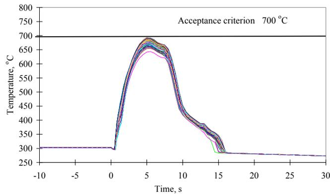
Fig. 5. Fuel cladding temperatures at the location of 2.75 m from the core bottom obtained using SUSA generated runs from RELAP5 calculations
