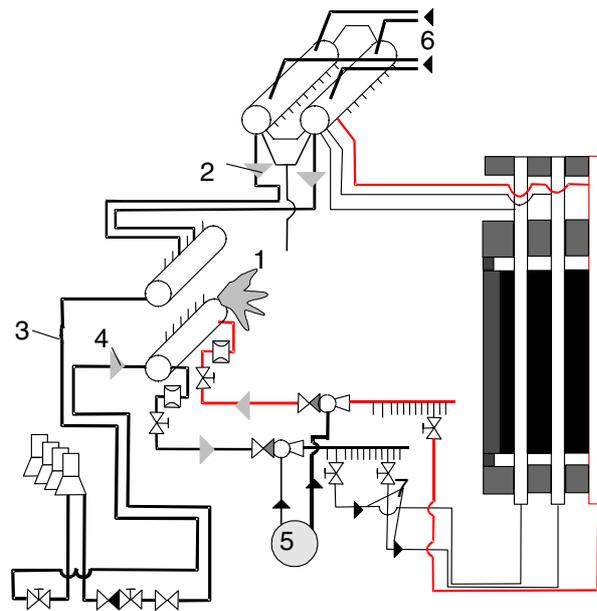
Fig. 1. MCP pressure header break with failure to close check valve of one GDH. Structure of coolant flows: 1 – break of PH; 2 – overflow of coolant from DS; 3 – MCP suction piping; 4 – coolant discharge from MCP pressure piping; 5 – ECCS water supply; 6 – steam supply from intact loop of the MCC; 7 – coolant supply into reactor core
