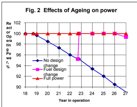
To counter these effects the life cycle management is in effect at all stations to monitor the extent of ageing degradation and ensures that corrective measures are implemented in a timely manner. However, the life cycle management may not be fully effective in countering the ageing effects and power derating may become a necessity in order to maintain adequate margins (Figure 2 illustrates the impact of ageing effects on the reactor power).
