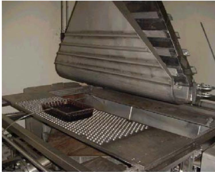
FIG. 1. Electron beam irradiation apparatus.
