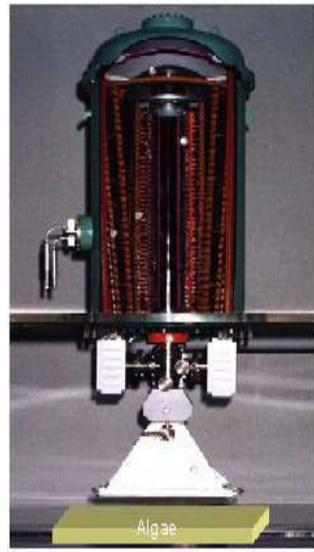
*FIG. 1. Schematic diagram of electron beam accelerator used for algae treatment*
