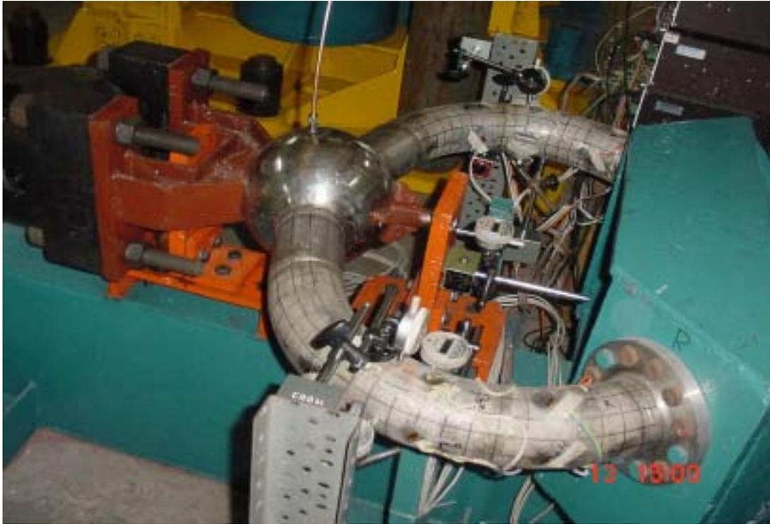
*FIG. 17. Ratchetting tests on a PSP model.*
