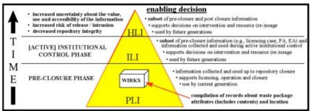
Fig. 1. Hierarchical Records for Radioactive Waste Management.
