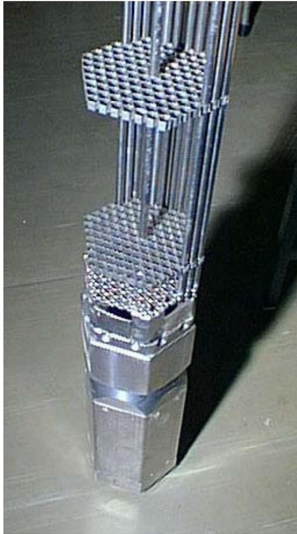
*FIG.III.1. Model of the fuel follower — absorber junction of a control assembly.*
