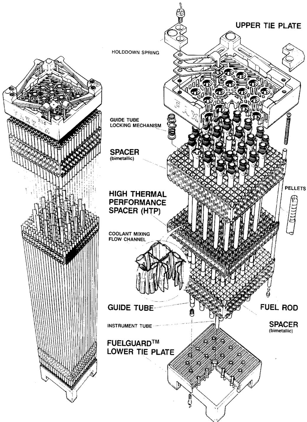
FIG. 6. Fuel assembly design for a PWR.
