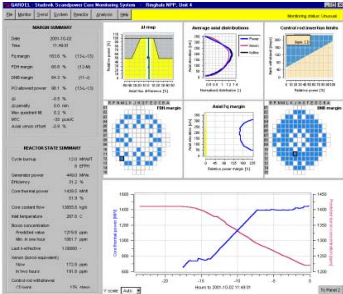
FIG. II.2. Example of screen available for the operator from the “GARDEL” CMS.
