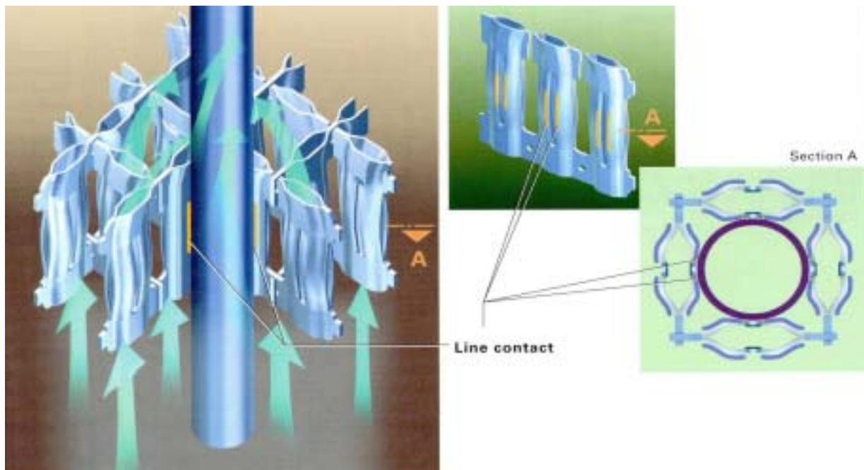
FIG. 7. High thermal performance (HTP) spacers.
