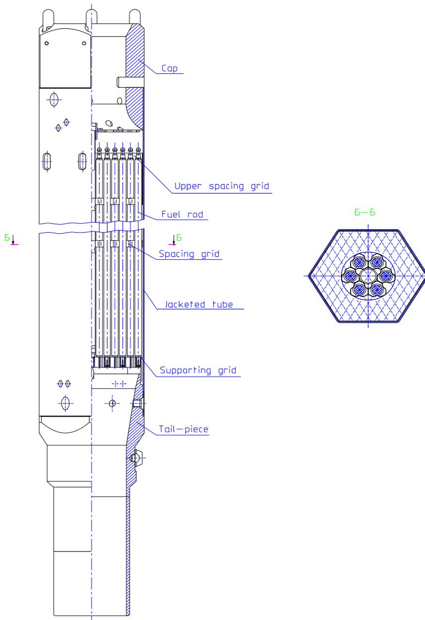
FIG. 2. The working assembly for a WWER-440.
