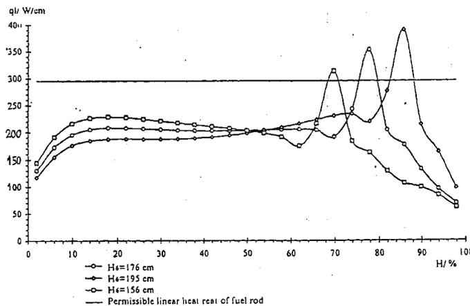
FIG. III.4. Distribution of linear heat rate over the height of fuel rod [1].
