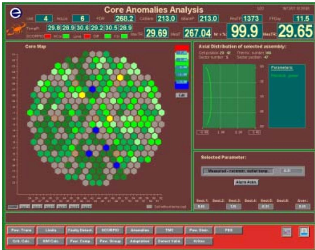
FIG. II.1. Example of screen available for the operator from the CMS.
