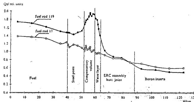
FIG. III.2. Distribution of relative heat rate over fuel rod height ( $Qz$ ) of working assembly adjacent to CPS working group [III.1].
