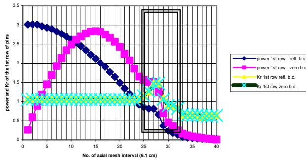
FIG. III.3. Axial dependence of the average power and radial power peaking Kr of the 1st row of pins for 3.82w% FA, boron zero [III.2].
