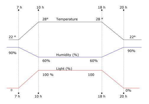
Figure 3.5. Environmental conditions of the wind tunnel.
