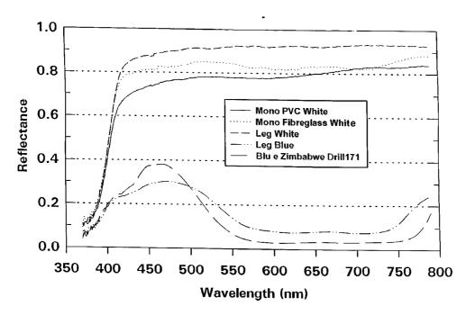
*Fig. 4.3. Reflectance of trap and target materials used for G. austeni monitoring and control.*
