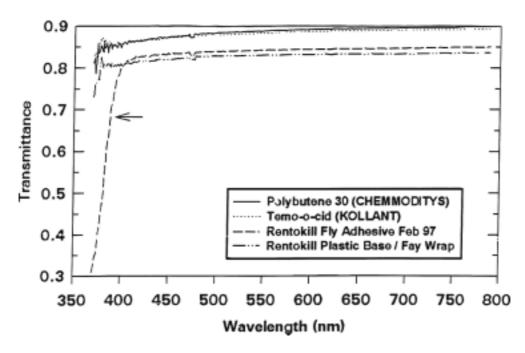
Fig. 4.4. Reflectance of adhesive materials used for G. austeni traps and targets.
