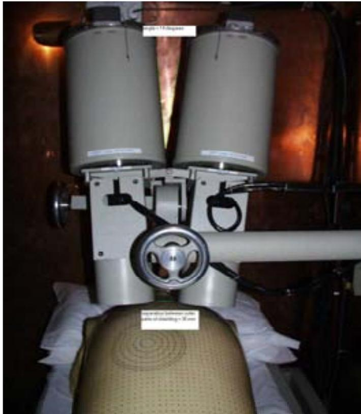
Fig. 1. Germanium detector array for lung counting (courtesy Australian Radiation Protection and Nuclear Safety Agency).
