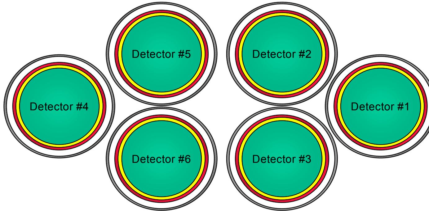
Note: Detectors 5&6 and Detectors 2&3 are two fixed assemblies
