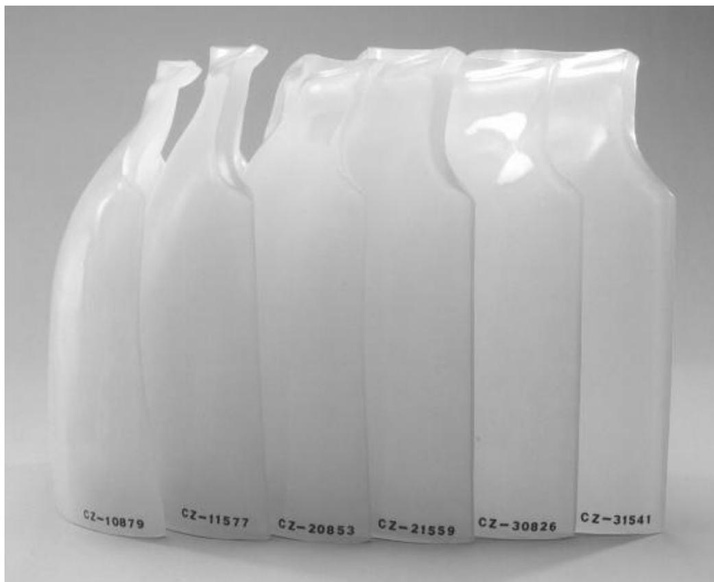
*FIG. 11. Chest overlays for JAERI phantom.*
