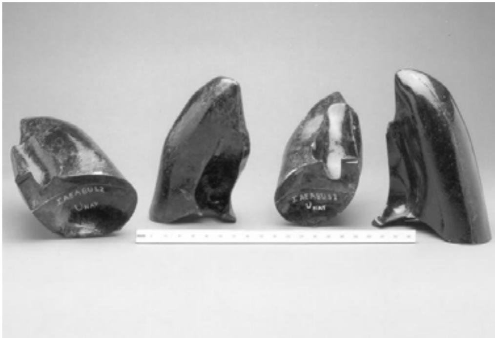
*FIG. 10. Natural uranium lung sets for JAERI phantom.*
