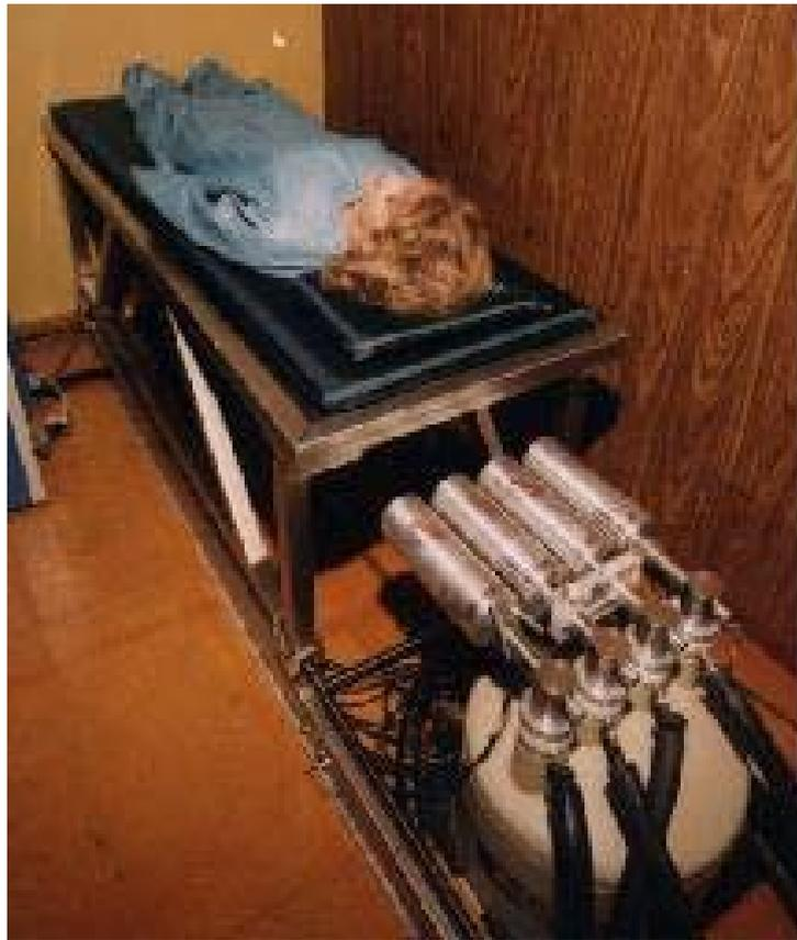
*FIG. 2. LLNL scanning bed whole body counter.*
