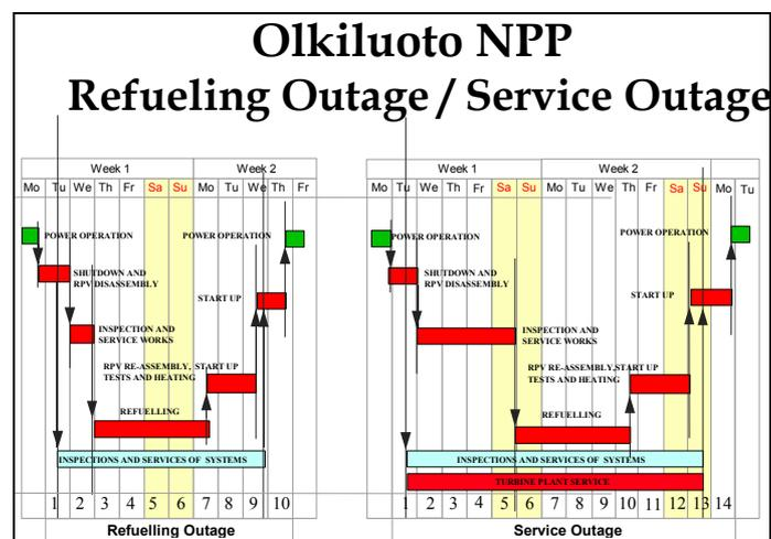
FIG. A.1. Olkiluoto nuclear power plant refueling/service outages.
