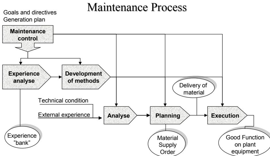
FIG. E.1. Maintenance process.
