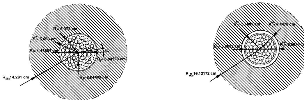
FIG. 17. Average cell for CAN NPP (A), and for CNE NPP (B).
