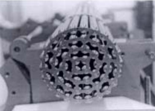
FIG. 8. Dismountable end plates of the CARA bundle with 52 fuel rods.
